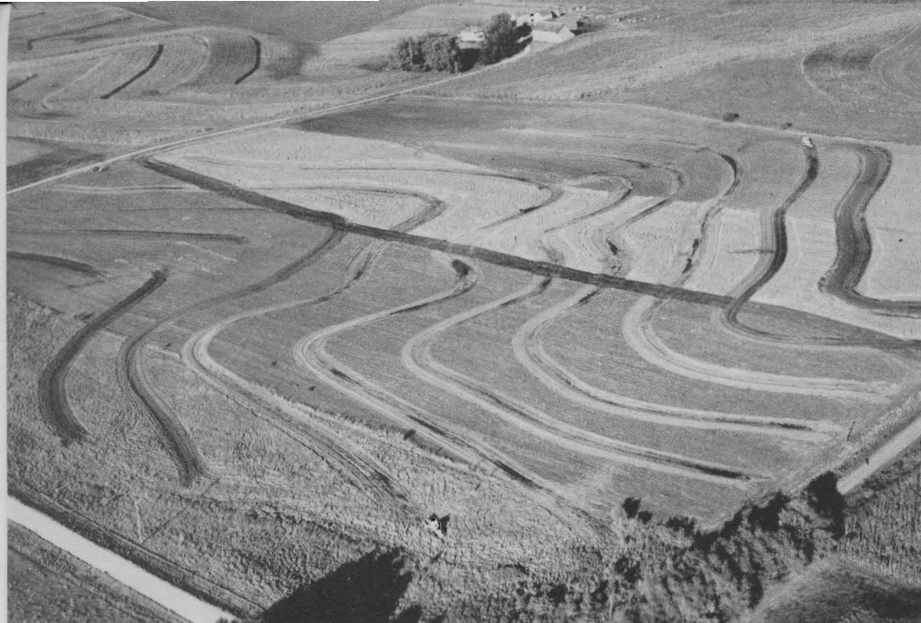
These standard terraces in southeastern Minnesota have a constant grade throughout their length, but spacing between adjacent terraces varies. This results in point rows which are difficult to farm and have become more of an inconvenience as the size of farm equipment has increased.
