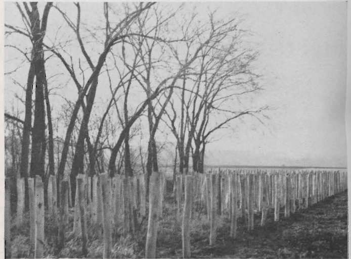
Fig. 1. Fenceposts are tested for durability in this plot on the University of Minnesota's St. Paul Campus.
