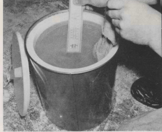
This insulated pail has a polystyrene liner and a metal outer jacket.
