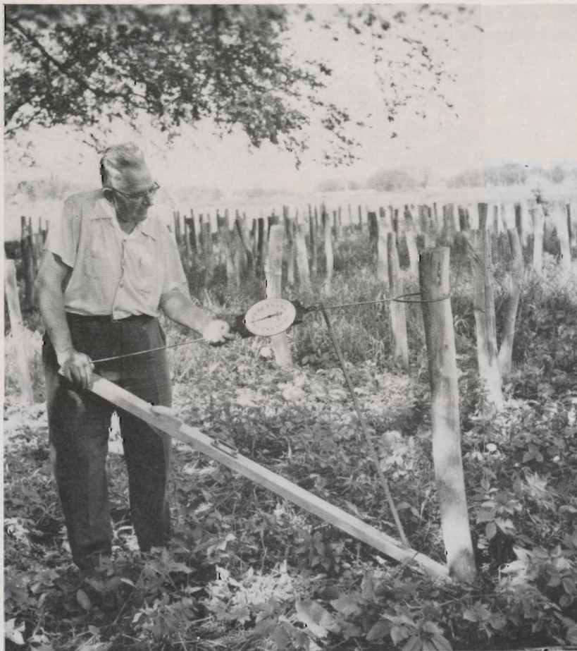
Fig. 2. J. R. Neetzel applies 100 pounds pressure to posts in test plot.
