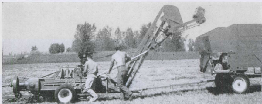
The experimental baler makes 12-inch cubic bales and moves the bales mechanically with an elevator into a trailing wagon.
