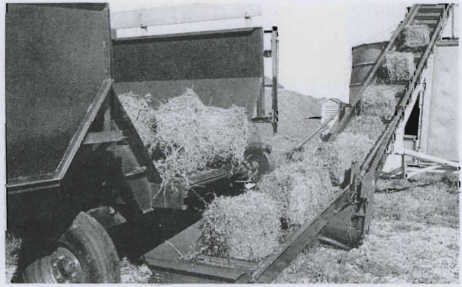
Small bales are easy to unload mechanically and elevate into a drying structure.
