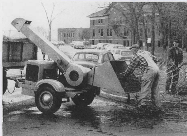
Fig. 2. Type of machine used for making wood chips from low-quality farm timber. Here it is being used to dispose of brush on the St. Paul Campus.
