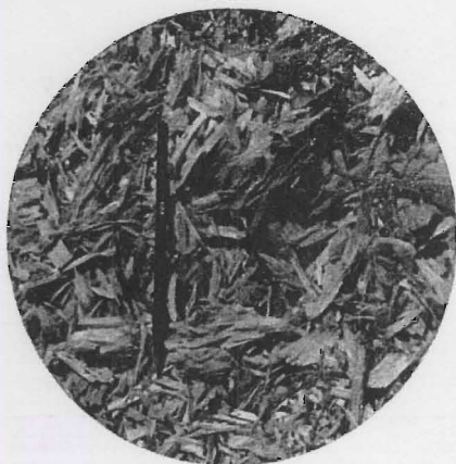
Fig. 1. Typical wood chips. The lead pencil gives an idea of their relative size.
