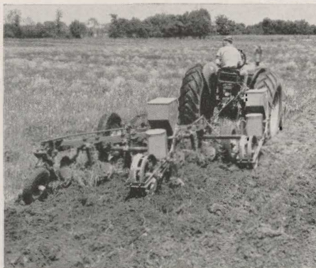
Fig. 2. "Plow-plant" means to plow and plant in one operation with seeders hitched to the plow. The implement here combines two planters with a 5-bottom plow.
