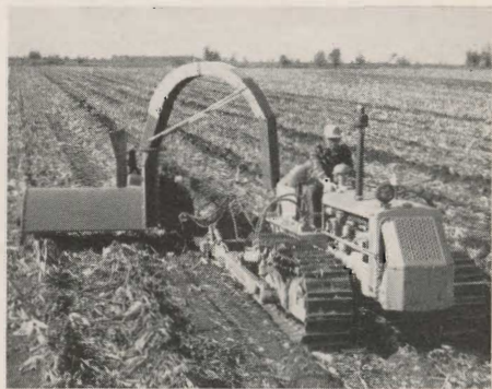
Fig. 7. This machine chops up plant residues and blows them into a deep chisel mark. Inventors call it "vertical mulching."
