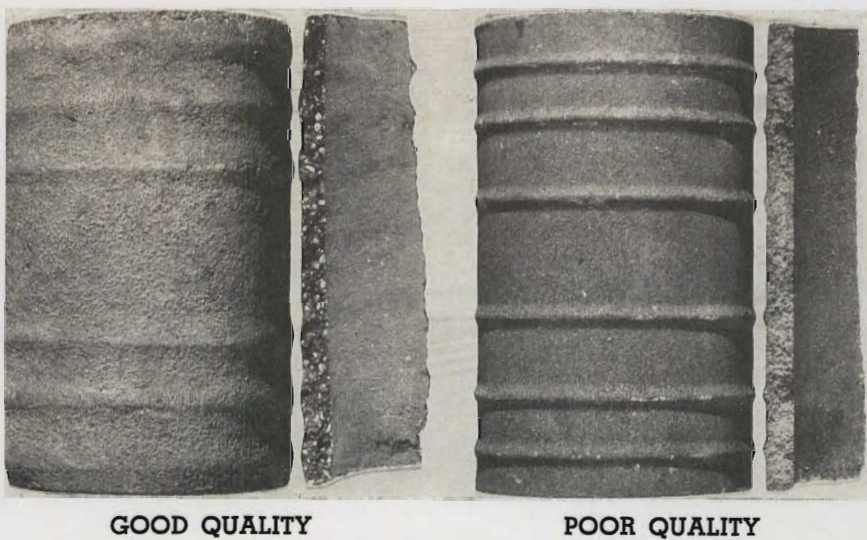
Fig. 1. Concrete drain tile of good and poor quality. Compare appearance of outside, inside, and broken edge of each tile.
