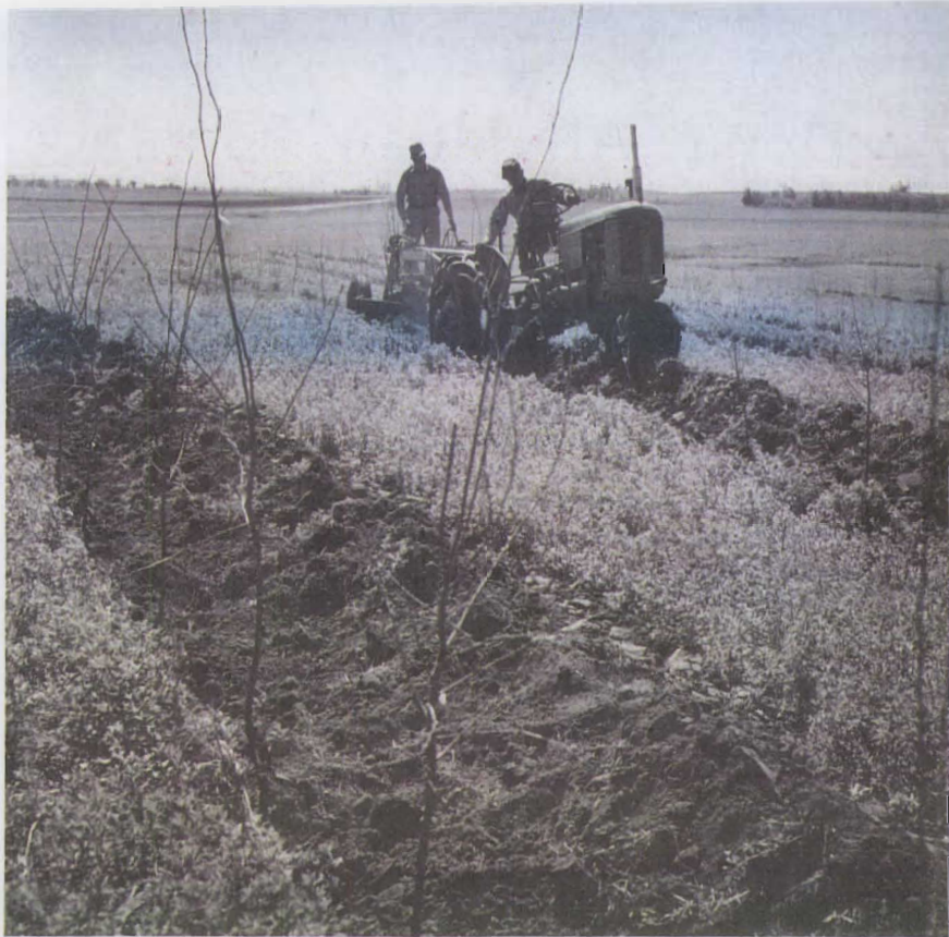
This tree-planting machine can plant an 800-foot, seven-row farmstead windbreak in two or three hours.
