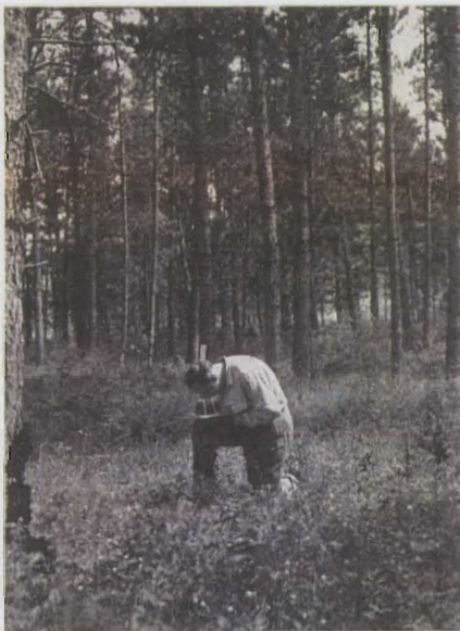
Checking the airphotos in the field. A pocket stereoscope is used here to check the accuracy of the mapping from aerial photographs in a 58-year-old jack pine stand.
