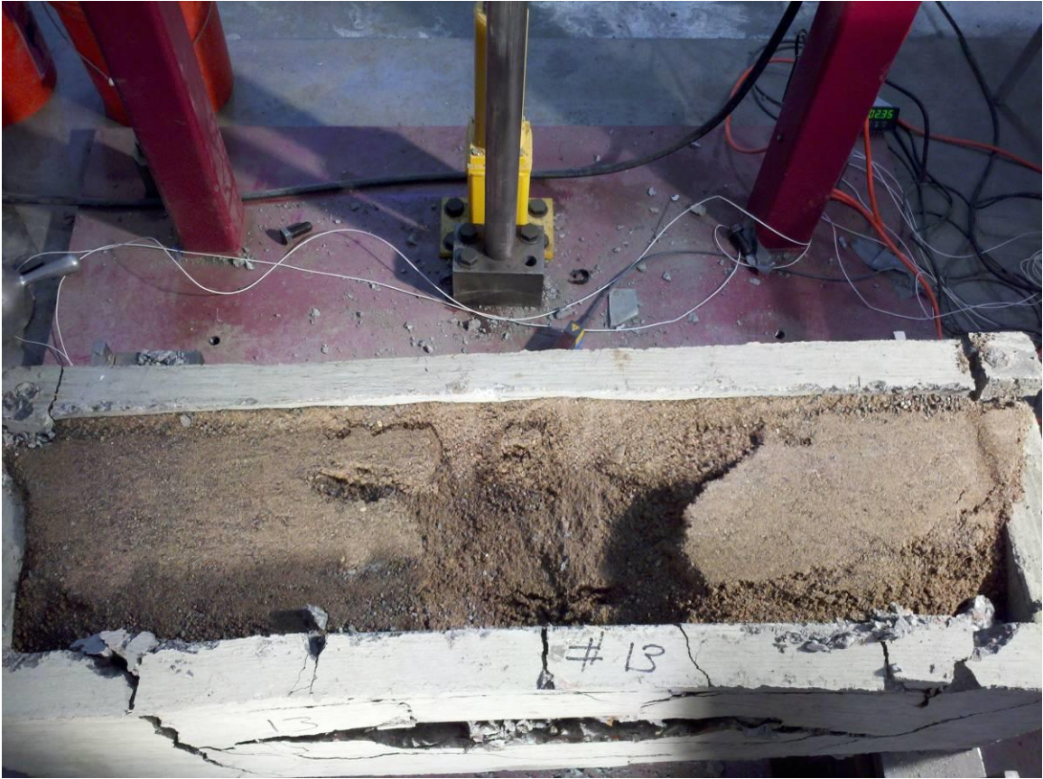
Fig 4-46 Test 13 – Sand Post-Impact
