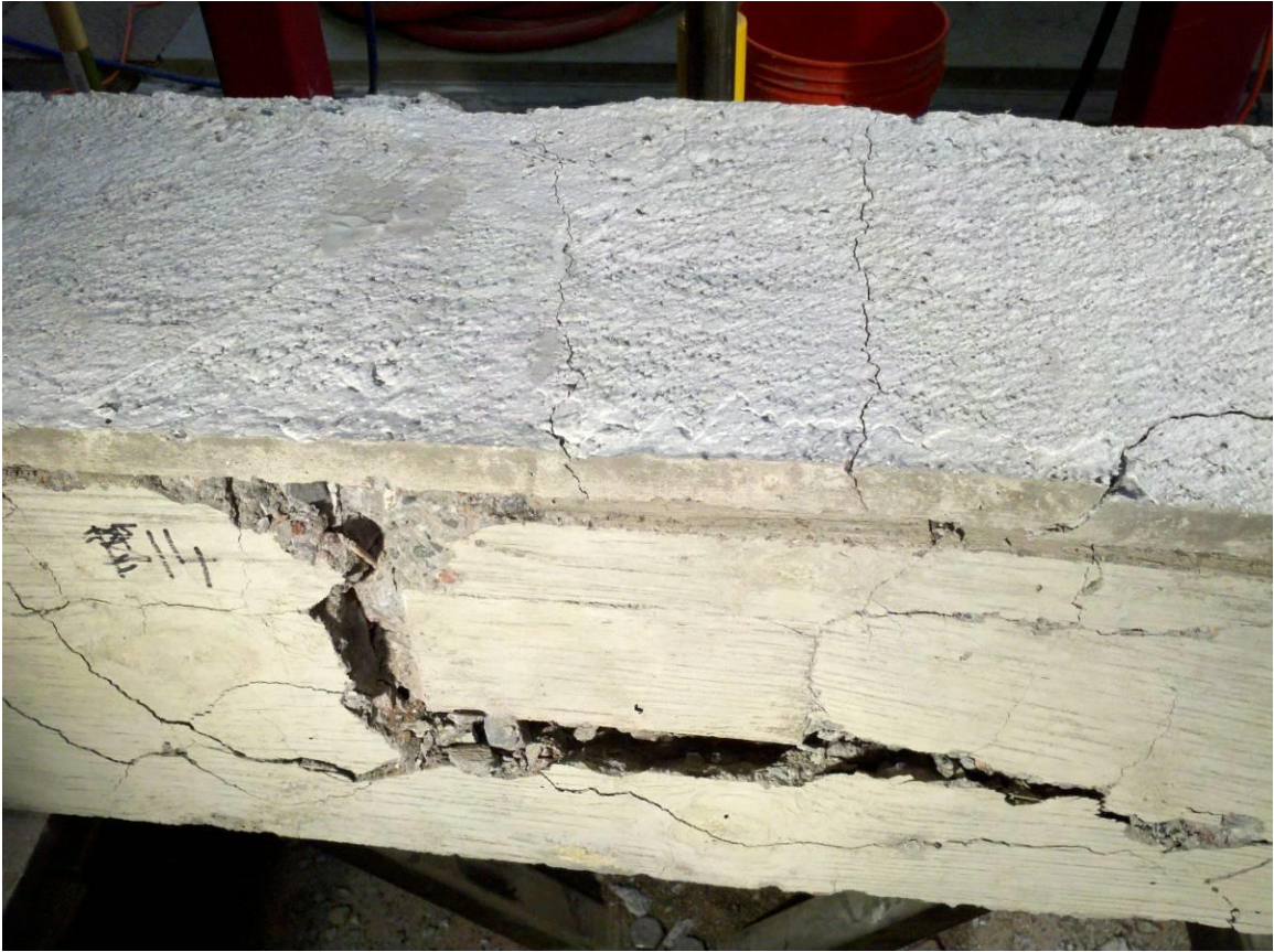
Fig 4-48 Test 14 – Plate Sand Compacted II Post-Impact
