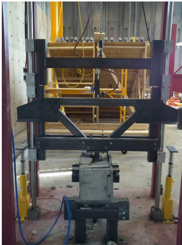
Fig 3-4 Impact carriage mounted below slave carriage in the machine on stainless steel rods
