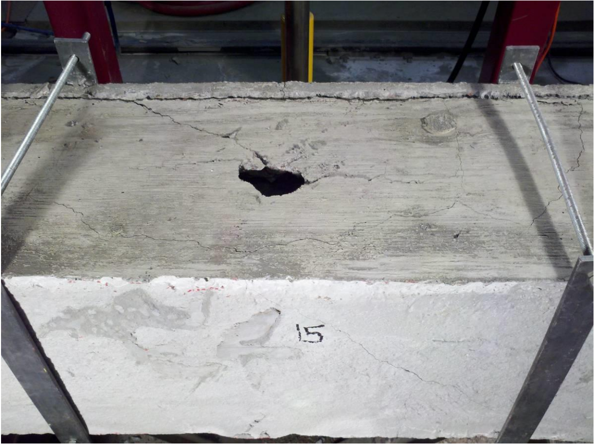
Fig 4-16 Test 15 – Side Penetration
