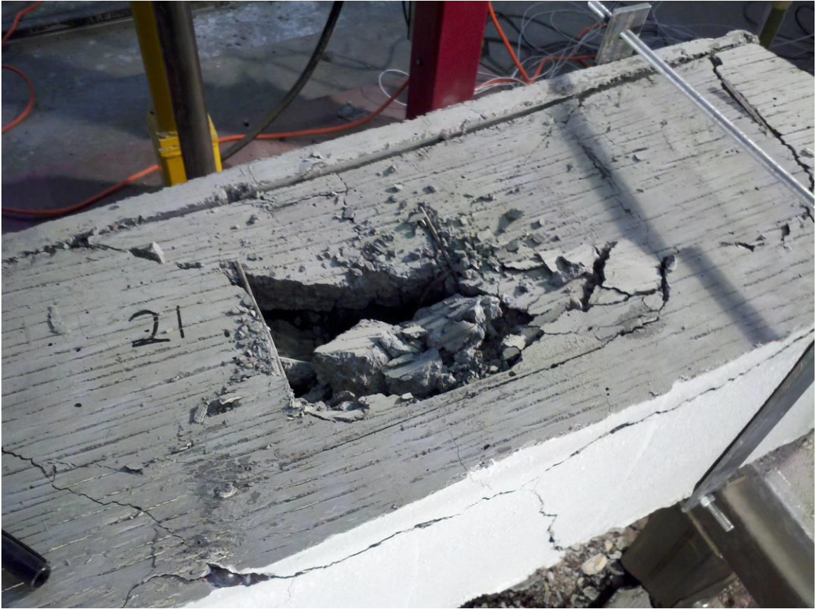
Fig 4-23 Test 21 – Round Soil Uncompacted II Post Impact
