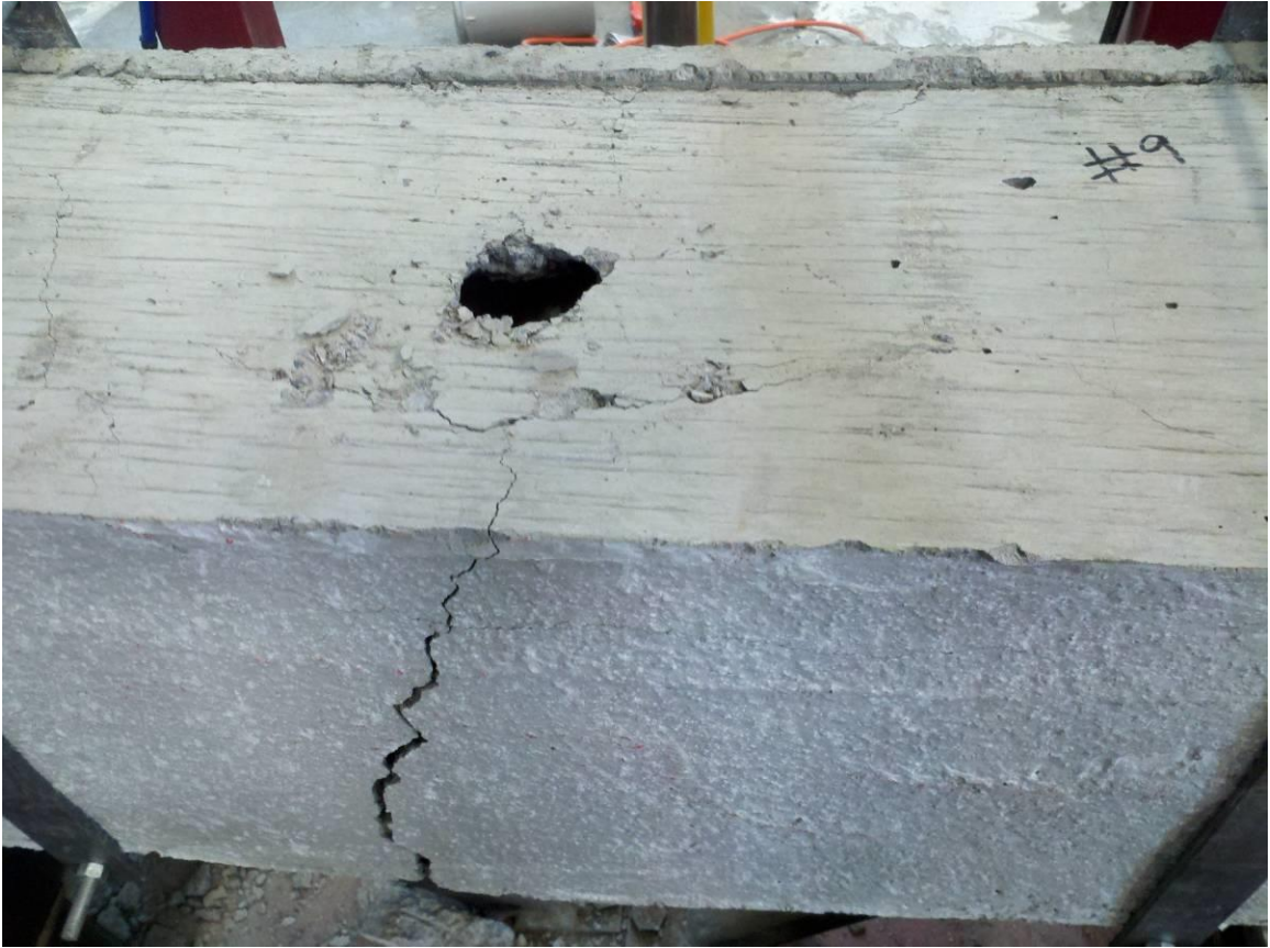
Fig 4-12 Test 9 – Round Sand Uncompacted II Post Impact
