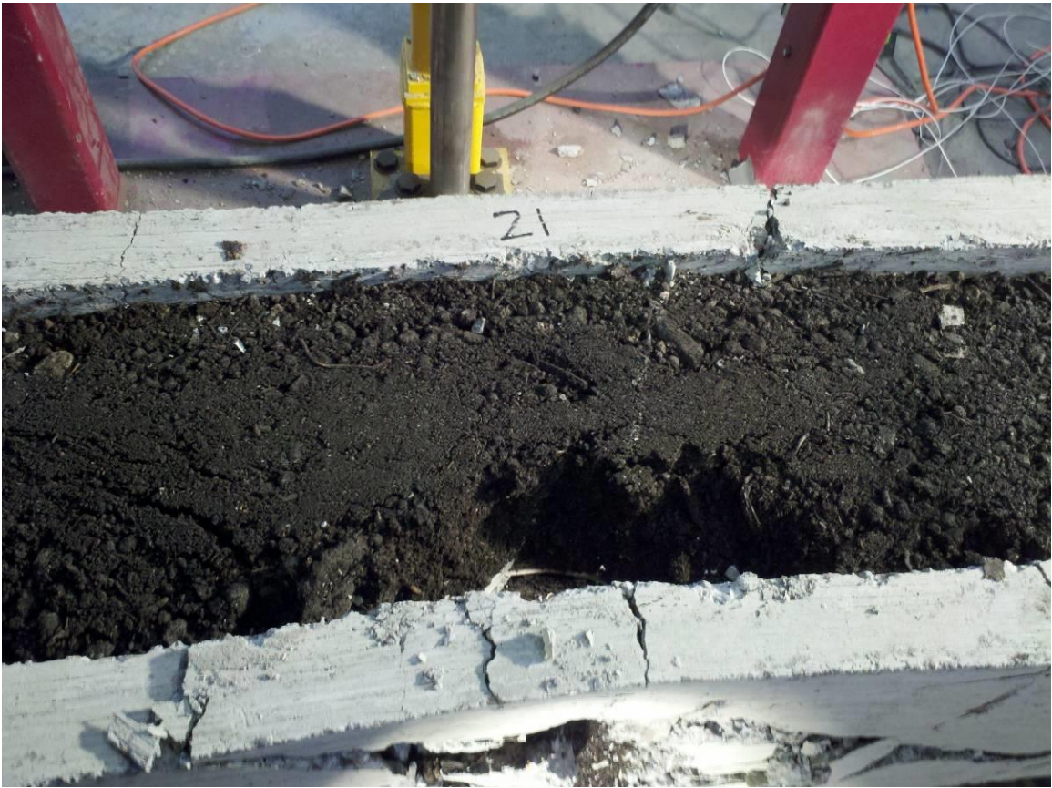
Fig 4-25 Test 21 – Soil Fill Post Impact
