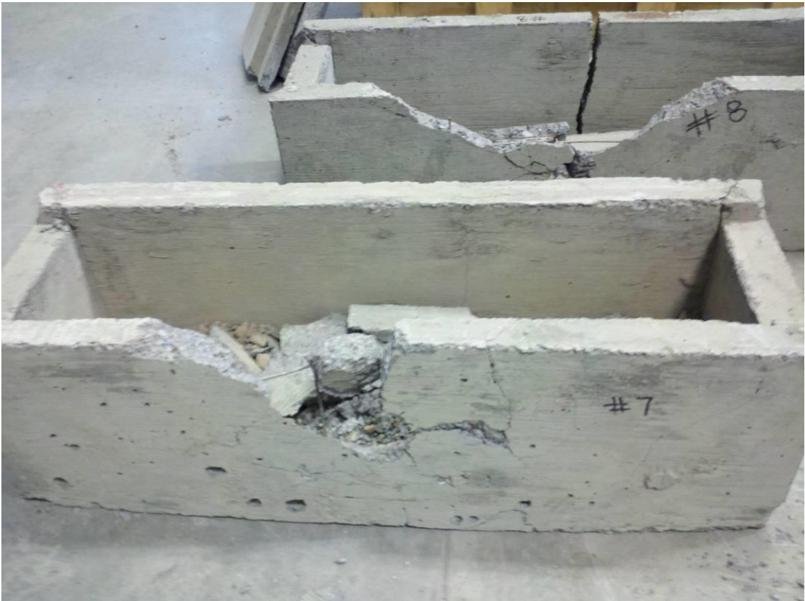
Fig 4-6 Test 7 - Round Coarse Aggregate 2 Post Impact
