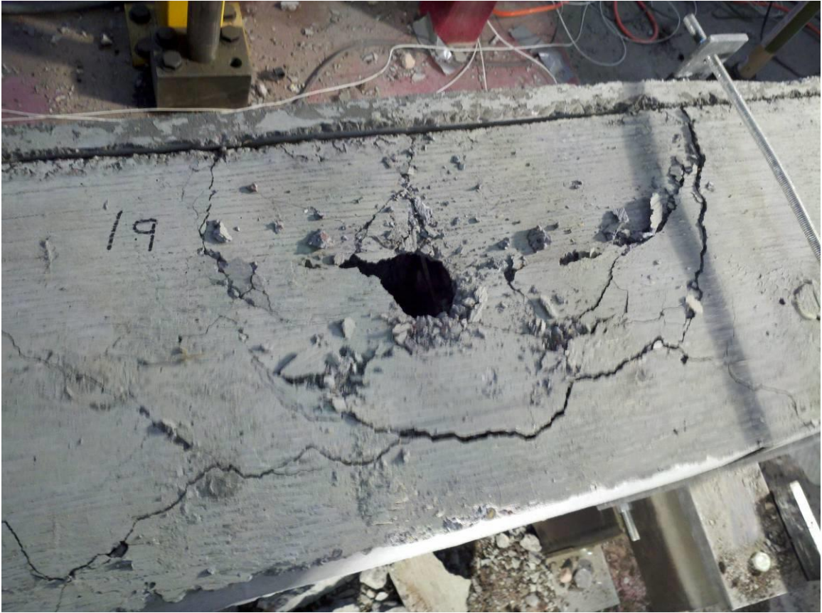
Fig 4-26 Test 19 – Round Soil Compacted I Post Impact
