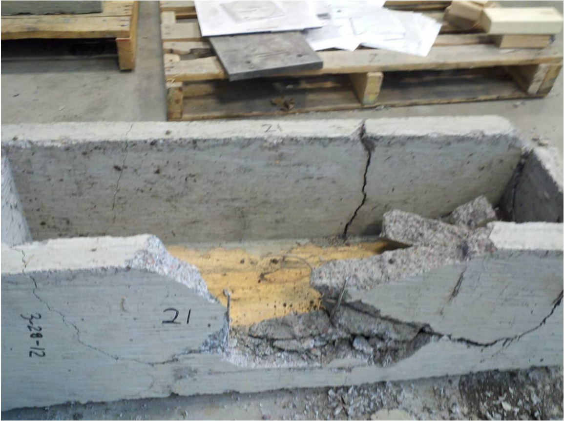
Fig 4-24 Test 21 – Emptied Post Impact
