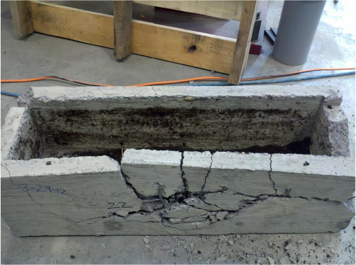
Fig 4-29 Test 22 – Round Soil Compacted 2 Post Impact
