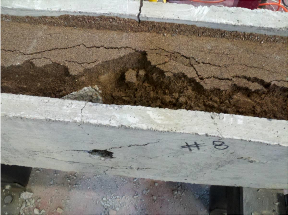
Fig 4-10 Test 8 - Round Sand Uncompacted I Post Impact 2
