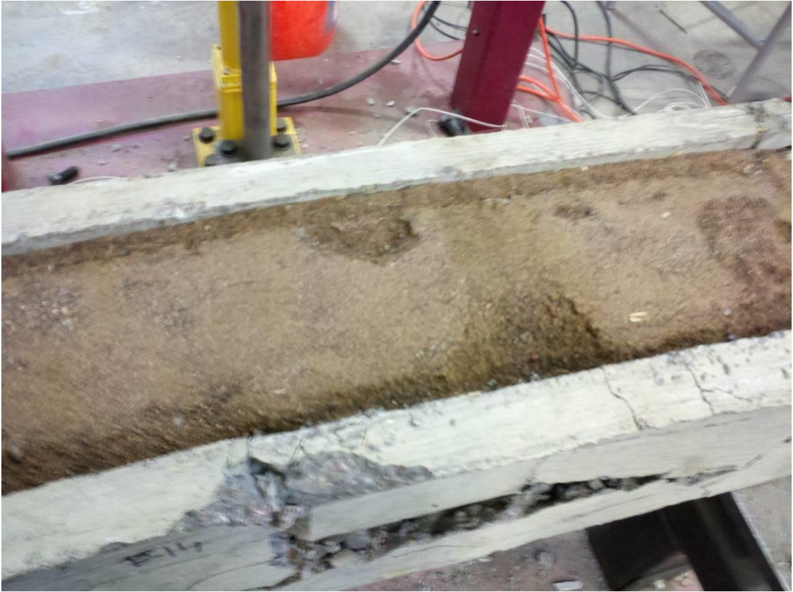
Fig 4-47 14 – Plate Sand Compacted II Sand Fill Post Impact
