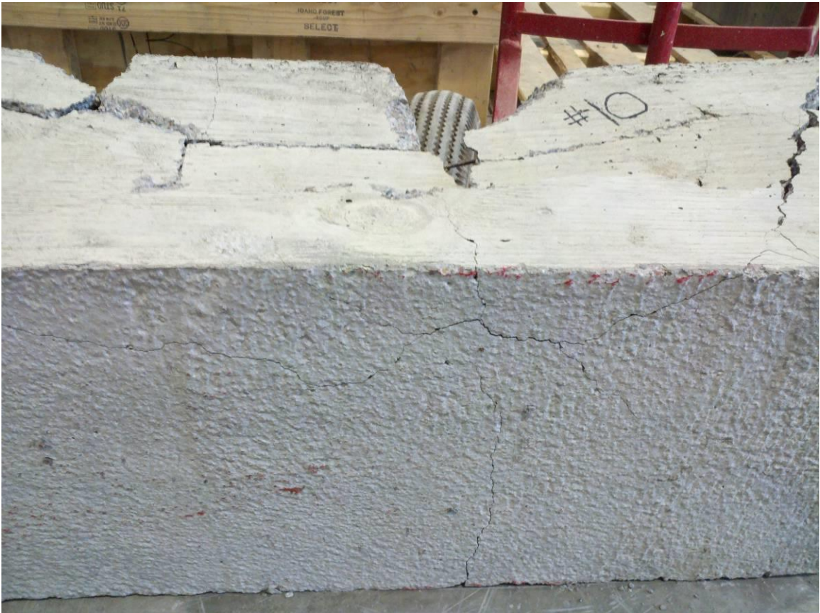
Fig 4-37 Test 10 – Plate Coarse Aggregate II Bottom Cracking
