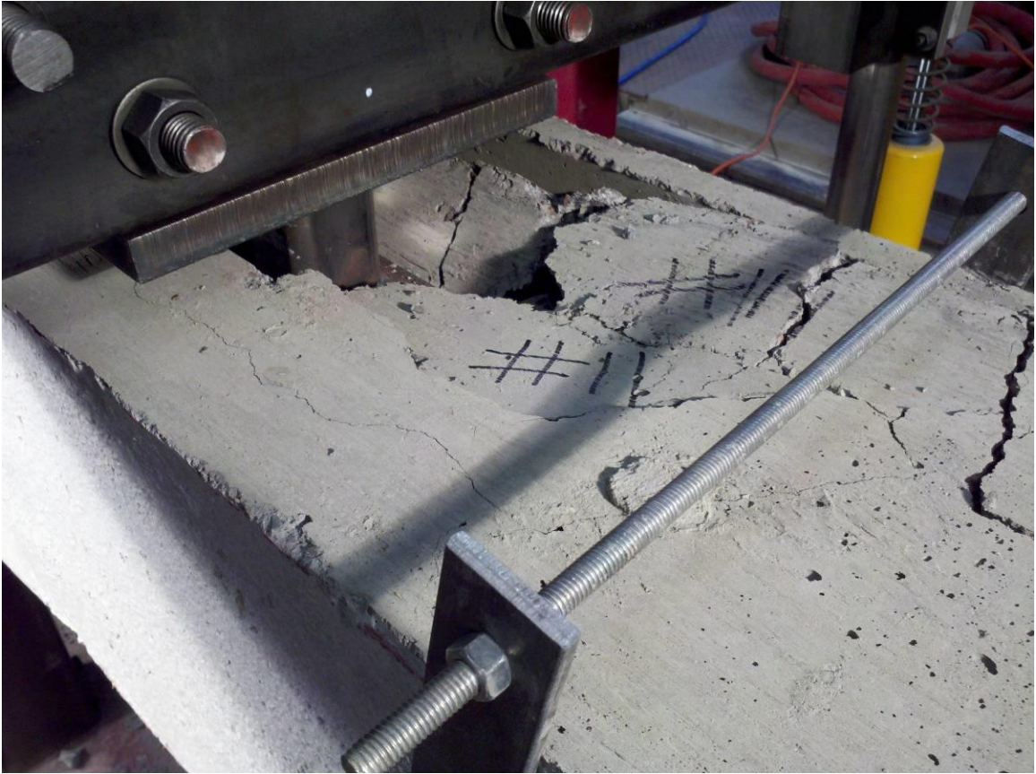
Fig 4-38 Test 11 – Plate Sand Uncompacted w/ Impactor Head
