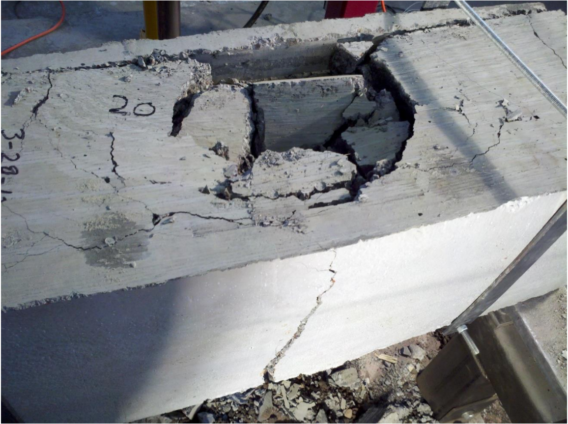
Fig 4-20 Test 20 – Round Soil Uncompacted I Post Impact
