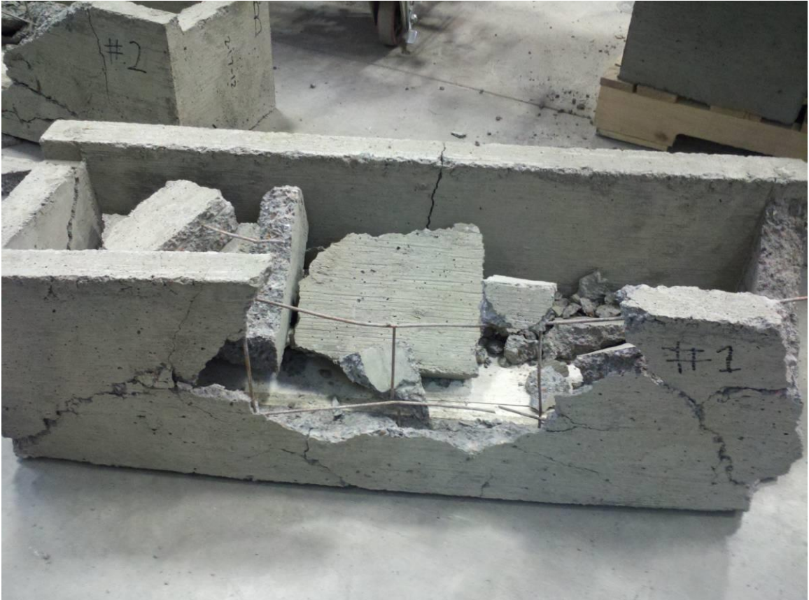
Fig 4-30 Test 1 – Plate Control I Post Impact
