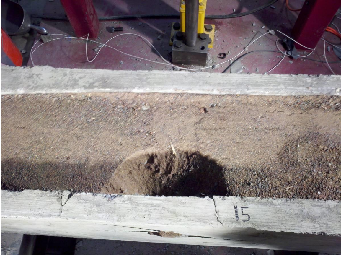
Fig 4-17 Test 15 – Sand Fill Post-Impact
