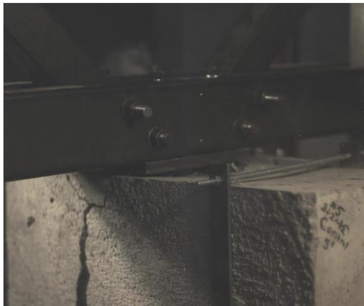
Fig 4-3.2 Test 5 – Carriage Impact from high speed footage
