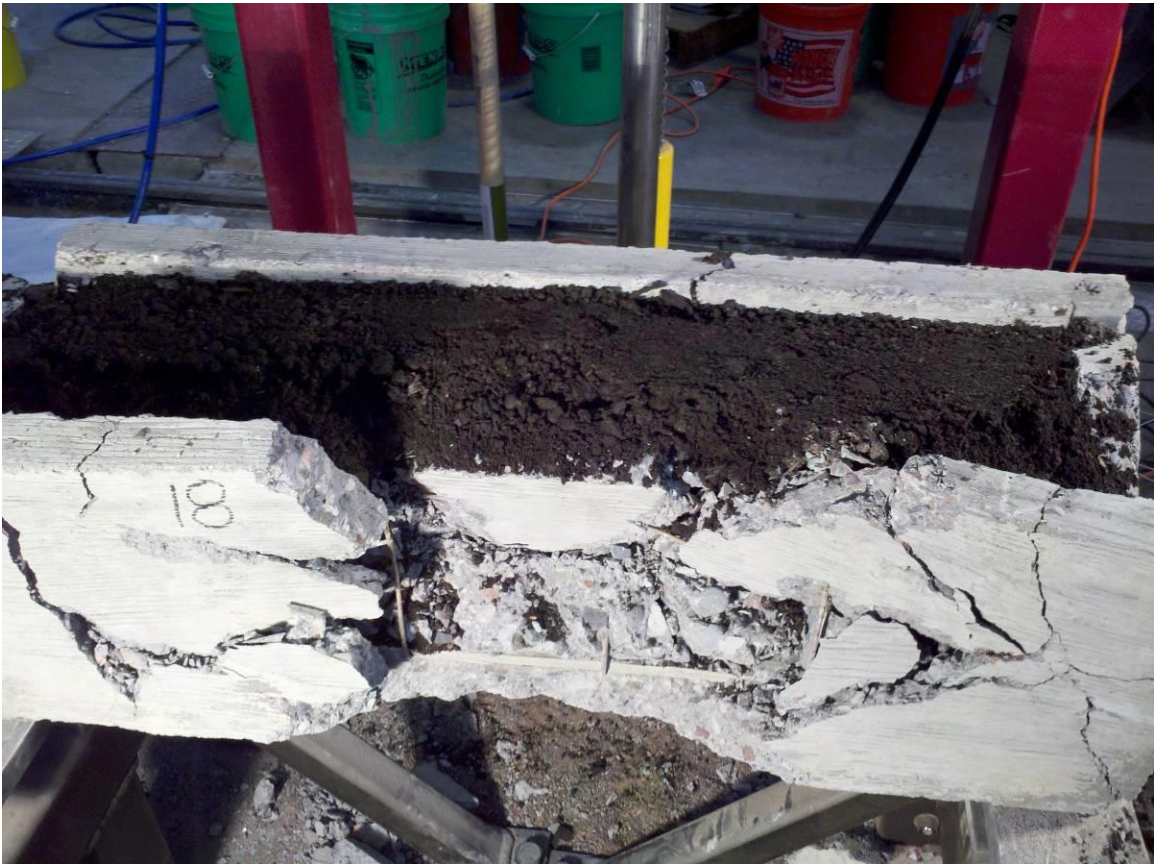
Fig 4-53 Test 18 – Plate Soil Uncompacted II Post Impact
