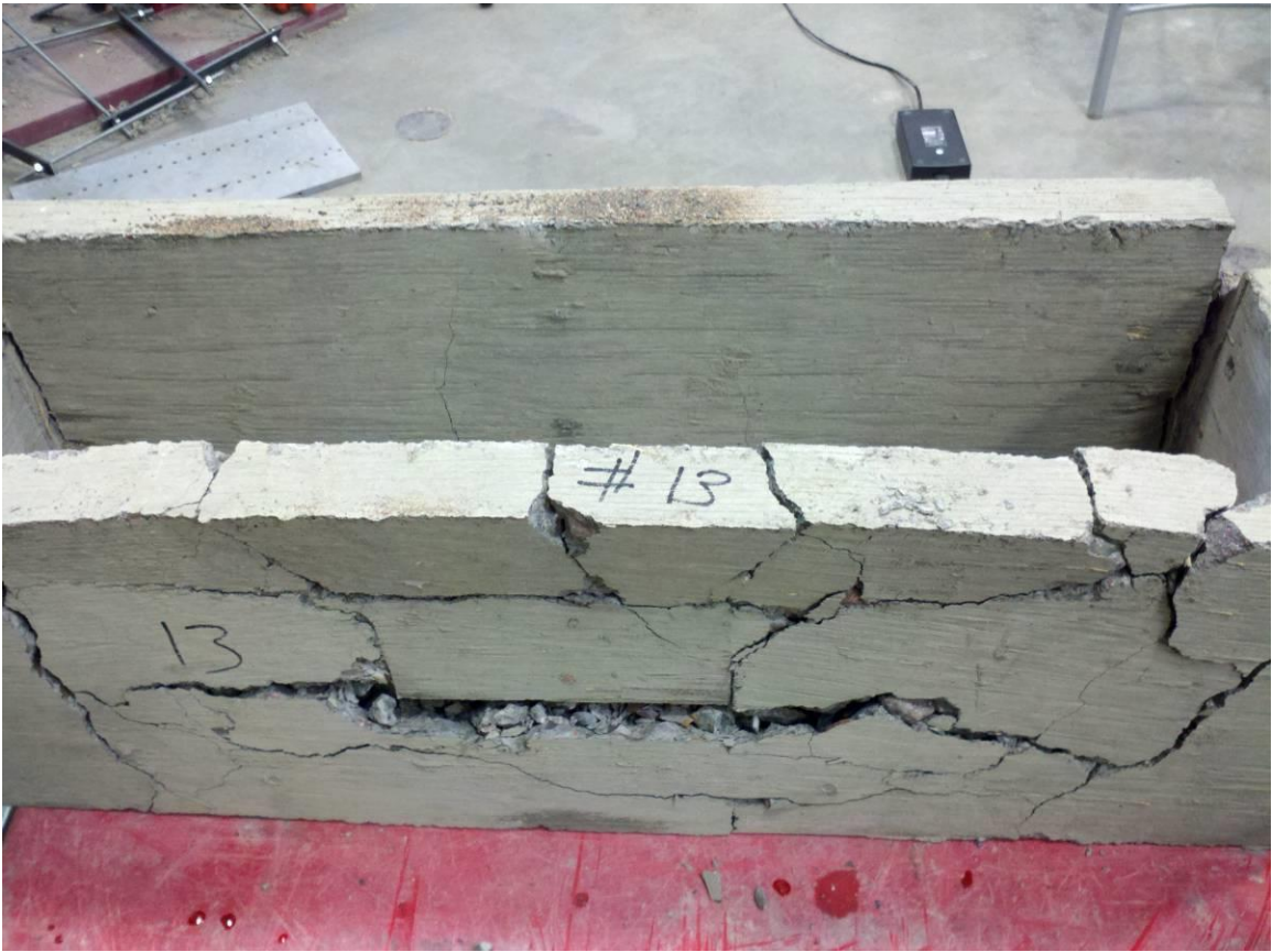
Fig 4-45 Test 13 – Plate Sand Compacted Emptied
