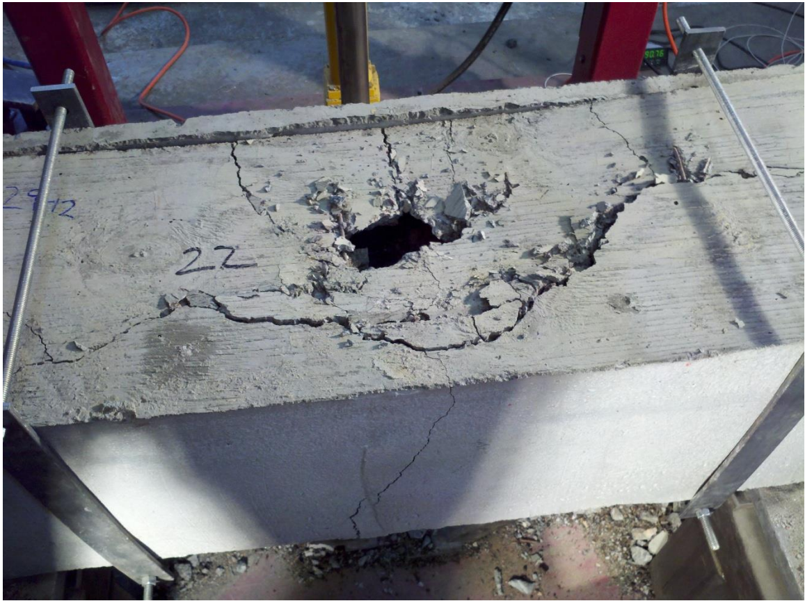
Fig 4-30 Test 22 – Side Hole Penetration
