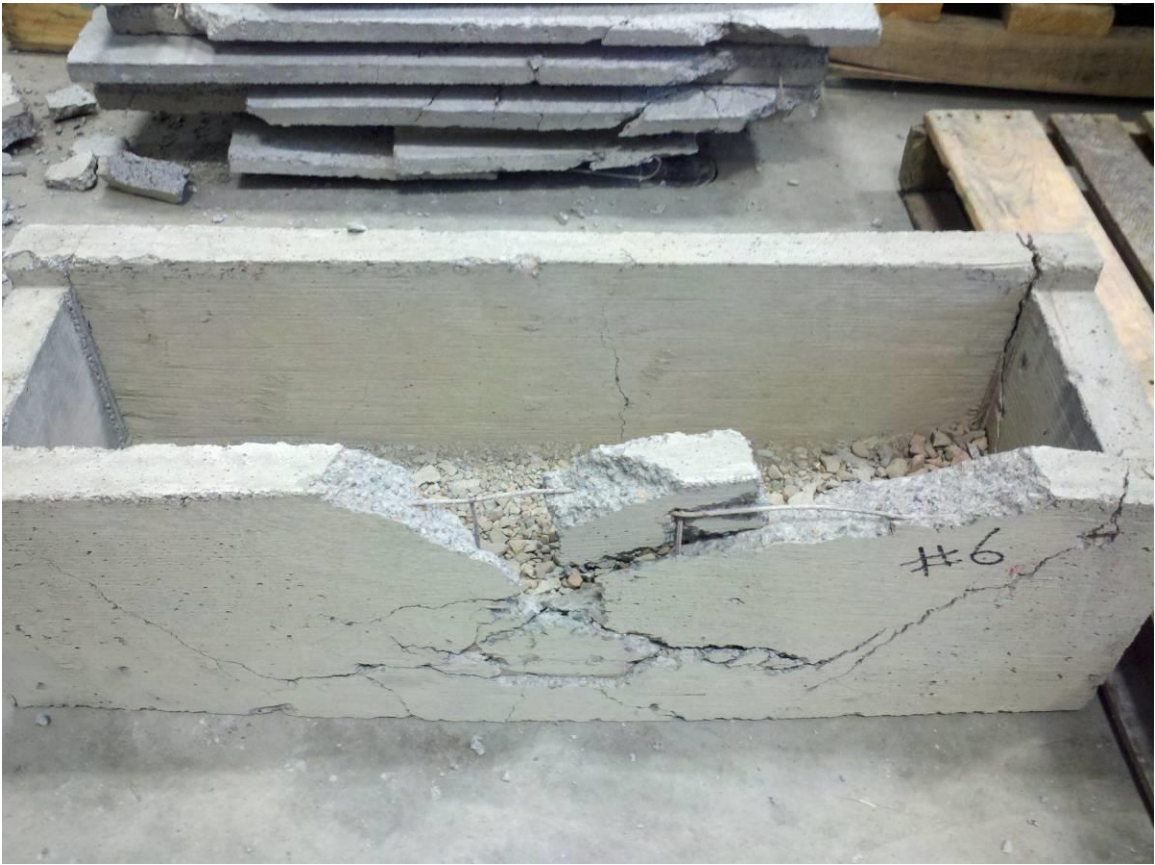
Fig 4-5 Test 6 - Round Coarse Aggregate I Post Impact
