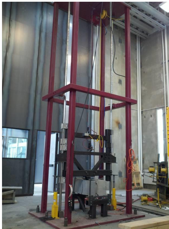
Fig 3-1 Impact testing machine with concrete box section in testing bay
