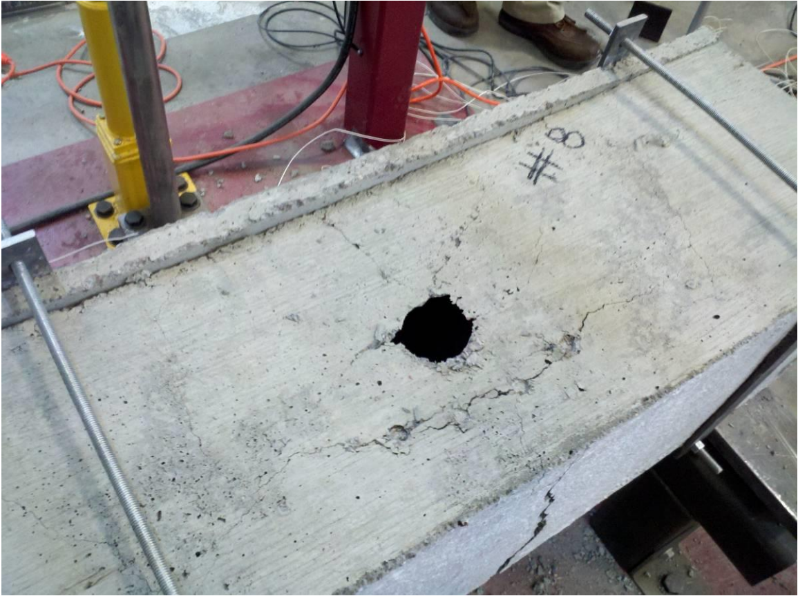
Fig 4-11 Test 8 - Round Sand Uncompacted I Post Impact Penetration
