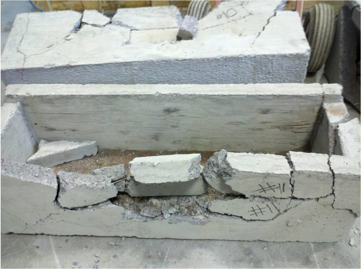
Fig 4-39 11 – Plate Sand Uncompacted Emptied
