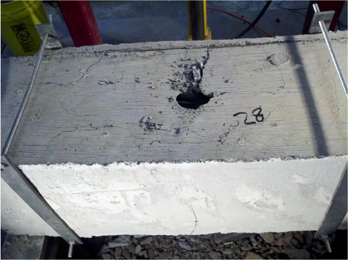
Fig 4-32 Test 28 – Round River Gravel II Post Impact
