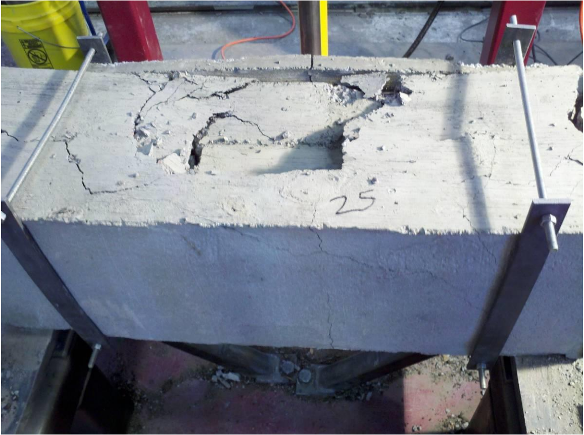
Fig 4-60 Test 25 – Plate River Gravel I Post Impact
