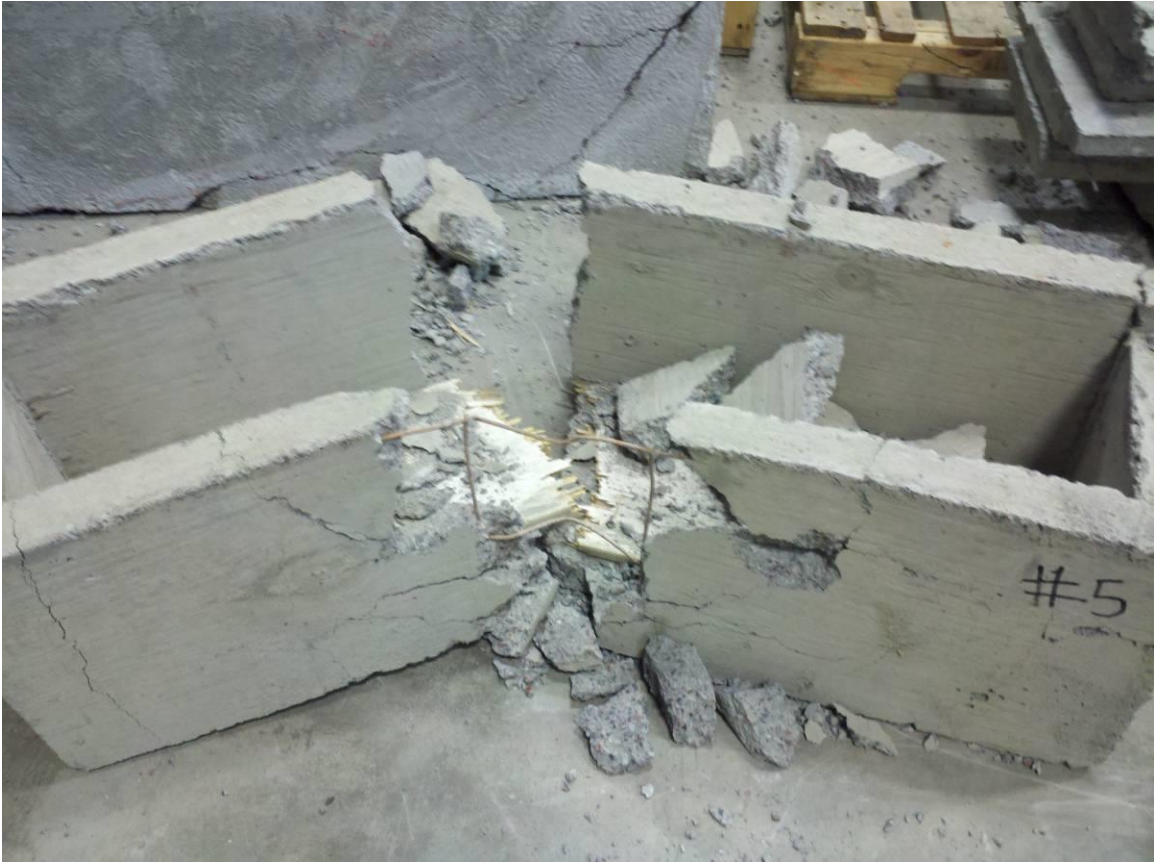
Fig 4-3 Test 5 - Round Control II Post Impact
