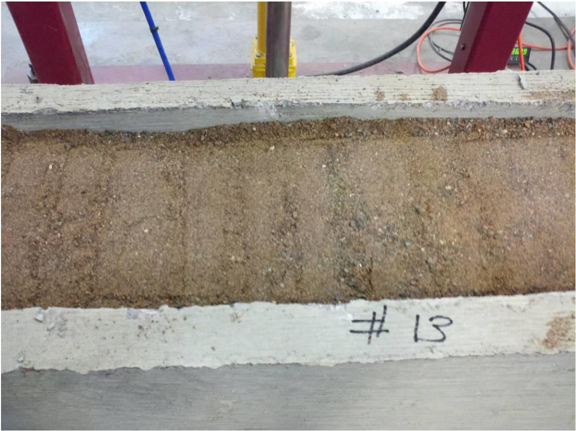
Fig 4-43 13 – Plate Compacted Sand Pre-Impact
