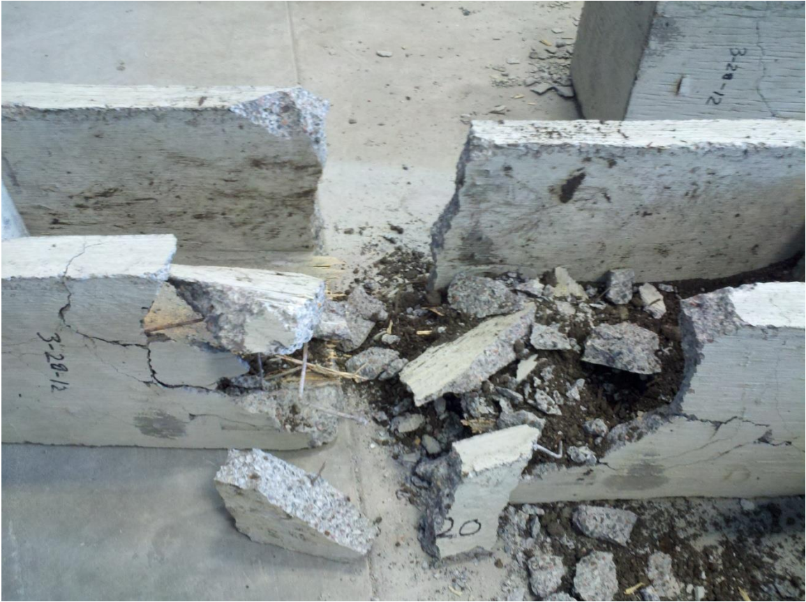
Fig 4-22 Test 20 – Emptied Post Impact
