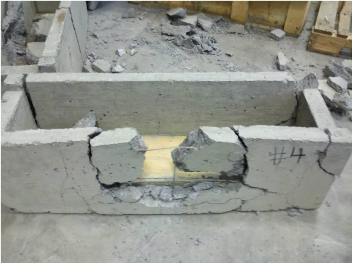
Fig 4-2 Test 4 - Round Control I Post Impact
