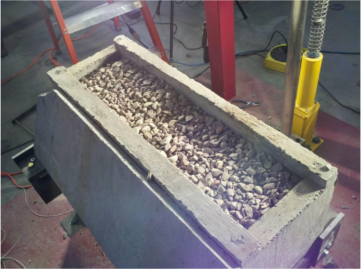
Fig 4-4 Round Coarse Aggregate Fill
