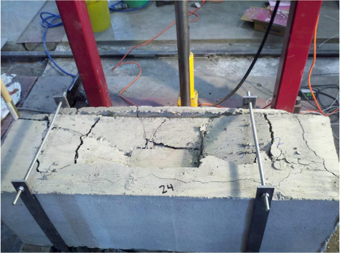
Fig 4-57 Test 24 – Plate Soil Compacted II Post Impact
