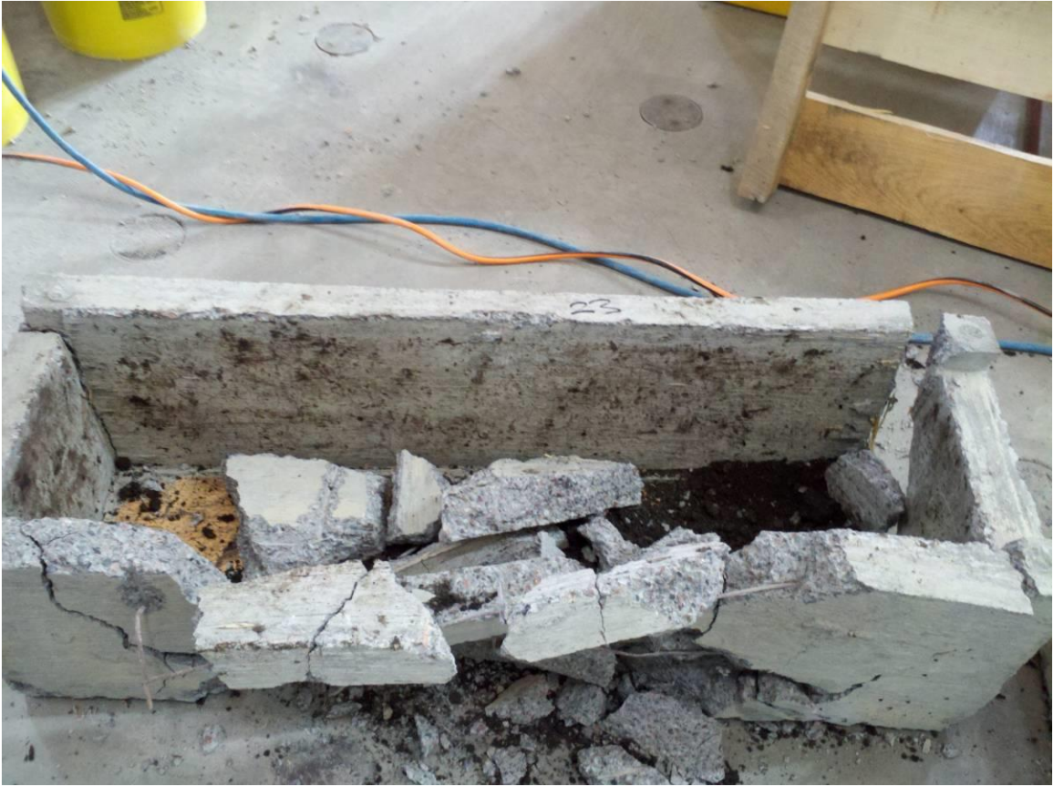
Fig 4-56 Test 23 – Plate Soil Compacted I Emptied
