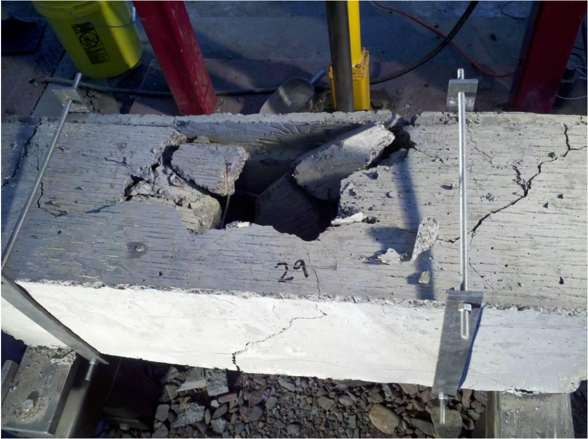
Fig 4-32 Test 29 – Plate Control III Post Impact
