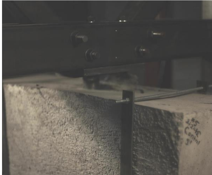
Fig 4-3.1 Test 5 – Impactor penetration from high speed footage
