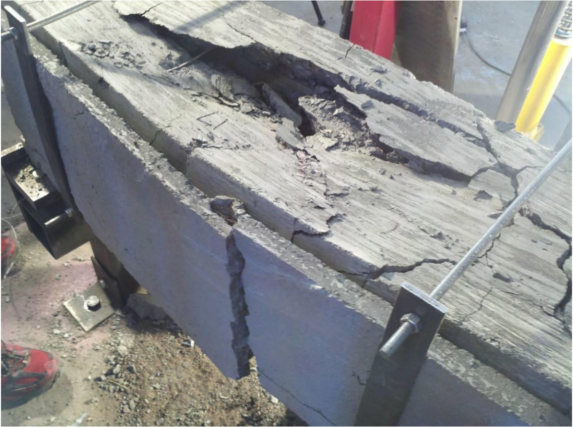
Fig 4-50 Test 17 – Plate Soil Uncompacted I Post Impact
