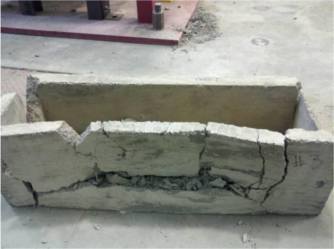
Fig 4-34 Test 3 – Plate Coarse Aggregate I Post Impact
