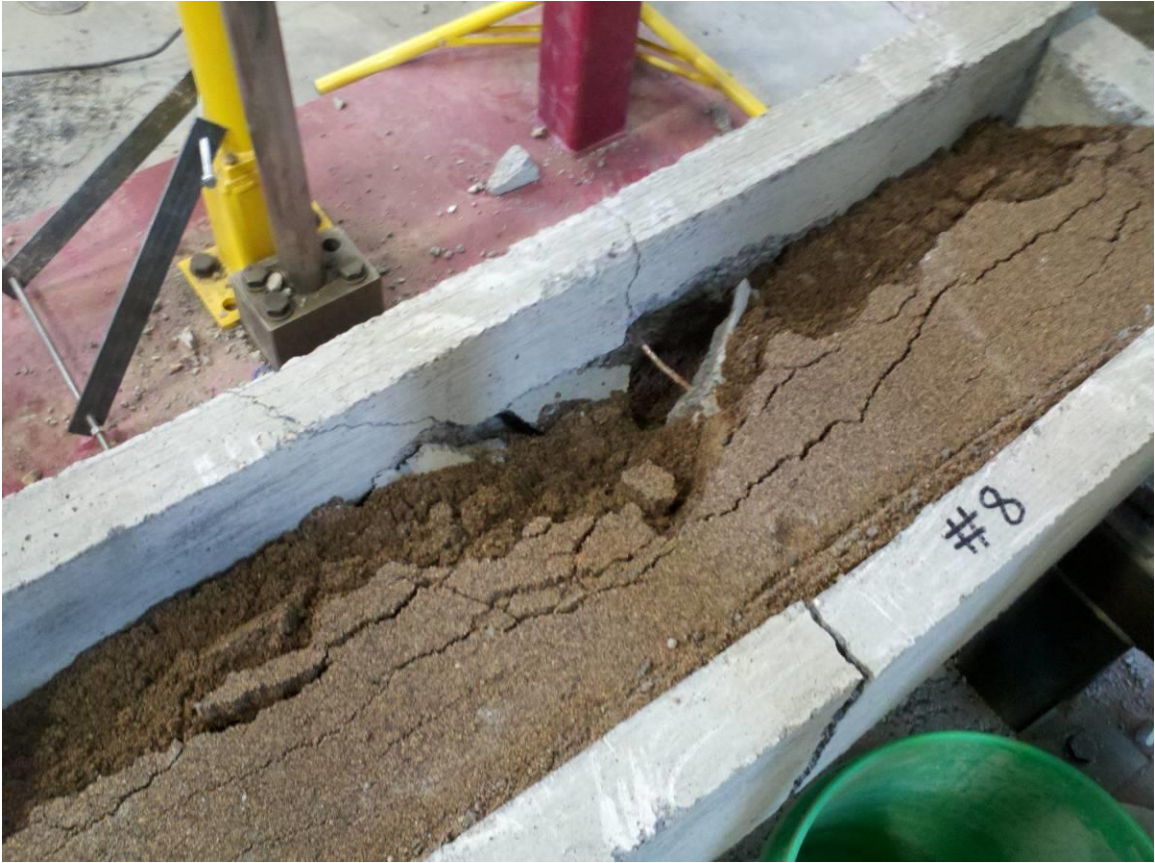
Fig 4-9 Test 8 – Round Sand Uncompacted I Post Impact
