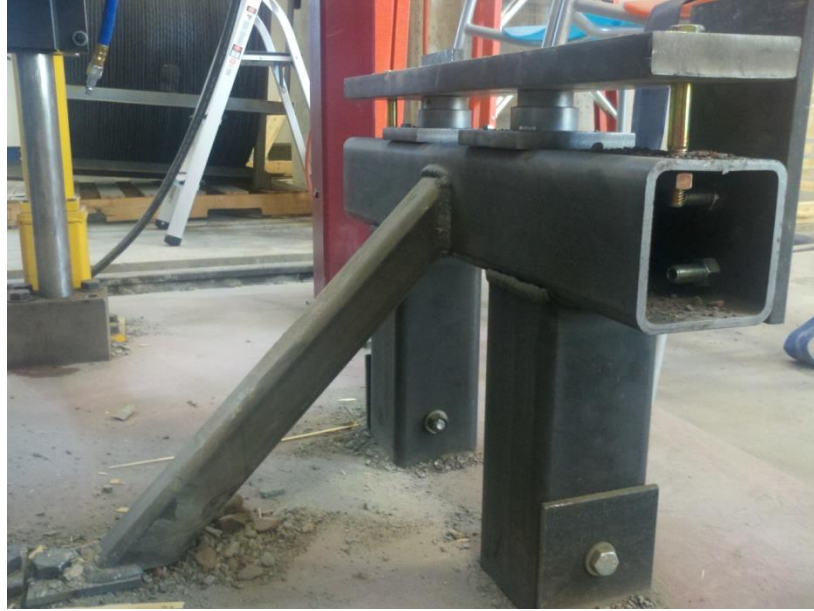
Fig 3-7 Load cell support setup
