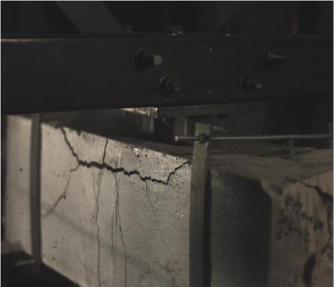
Fig 4-54 Test 17 – Plate Soil Uncompacted I Bottom Cracking
