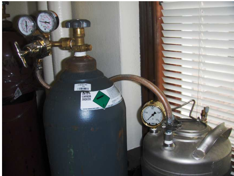
Figure 3.8: Pressure chamber and gauge used in calibrating the silicone tubing gas pressure samplers (Figure 3.9).
