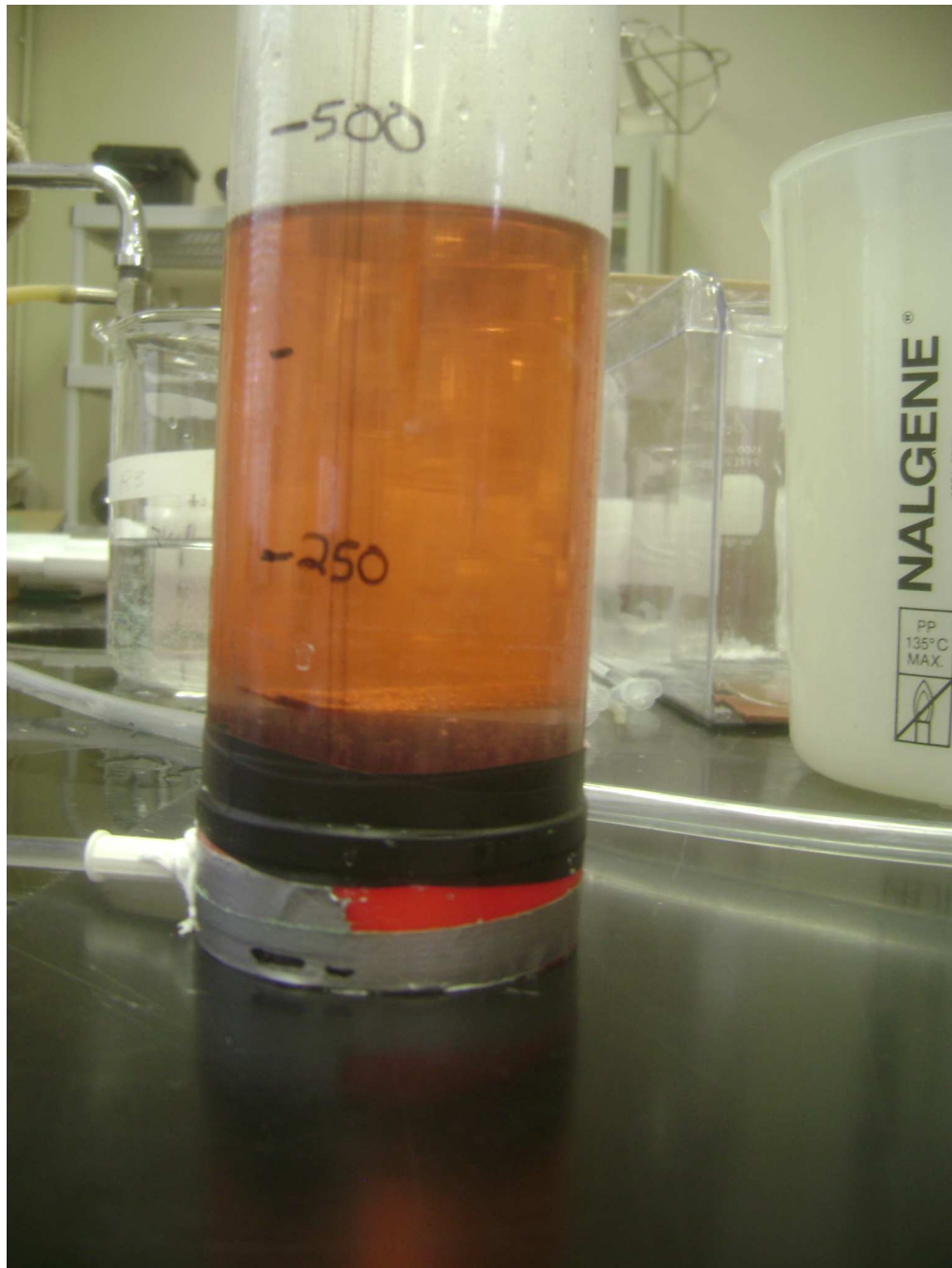
Figure 3.11: View of the bottom half of the tall narrower cylinder used to replace the beaker initially used in attempts to create a small scale limnic eruption.
