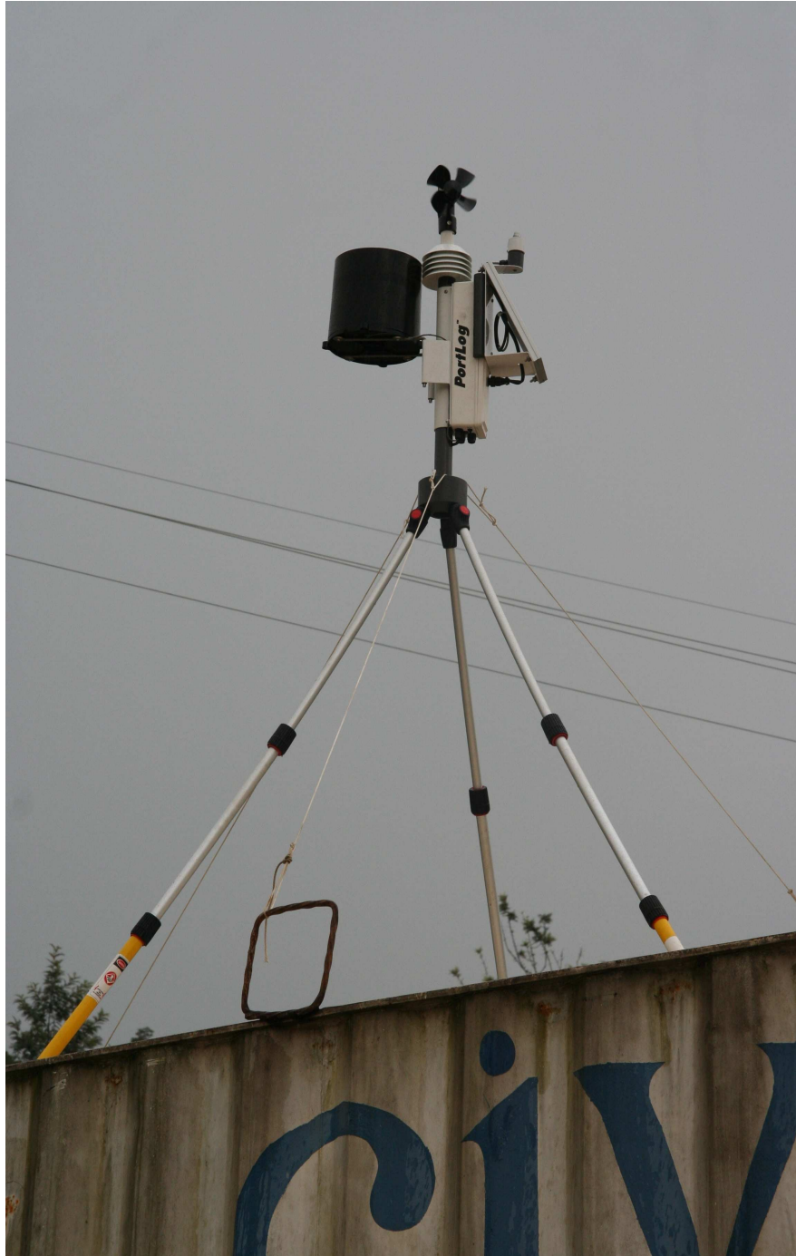
Figure 3.7: PortLog portable weather station installed near Kibuye, Rwanda.
