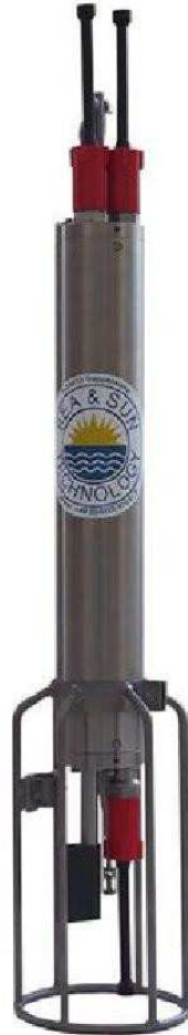
Figure 3.2: The Sea and Sun CTD 90M probe used to obtain profiles of temperature, conductivity, and dissolved oxygen concentration in Lake Kivu.
