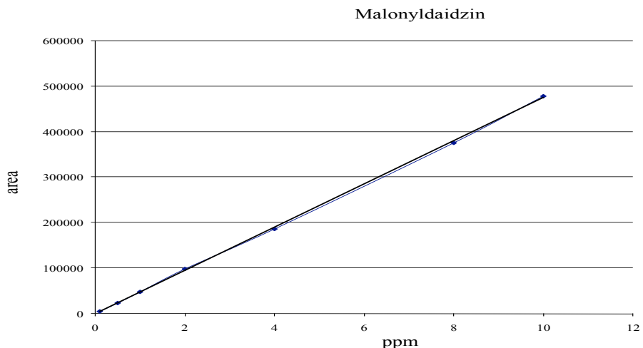
Figure 42. Calibration curve for malonyldaidzin with area (of the peak from HPLC analysis) on y-axis and concentration (in ppm) on x-axis. The line equation obtained after performing simple linear regression analysis of the data was: y = 47502x - 107.47 with R^2 value of 0.99.
