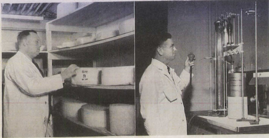
(Left) Professor Combs believes that research in cheese manufacture will give new outlets for Minnesota milk. (Right) Dr. Coulter demonstrates apparatus which will determine the percentage of oxygen in a sealed can of dried milk.
