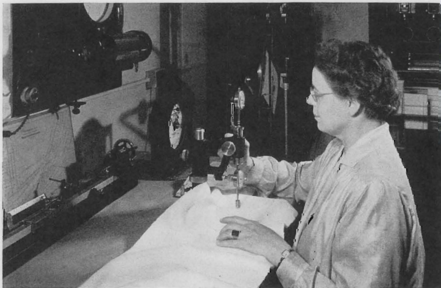
In the textiles laboratory of the Home Economics Division, Miss Phelps uses a compressometer to measure thickness and resilience of a wool blanket. Here also are instruments for measuring strength, weight, and abrasive resistance of fabrics, and the size, strength, and twist of yarns.
