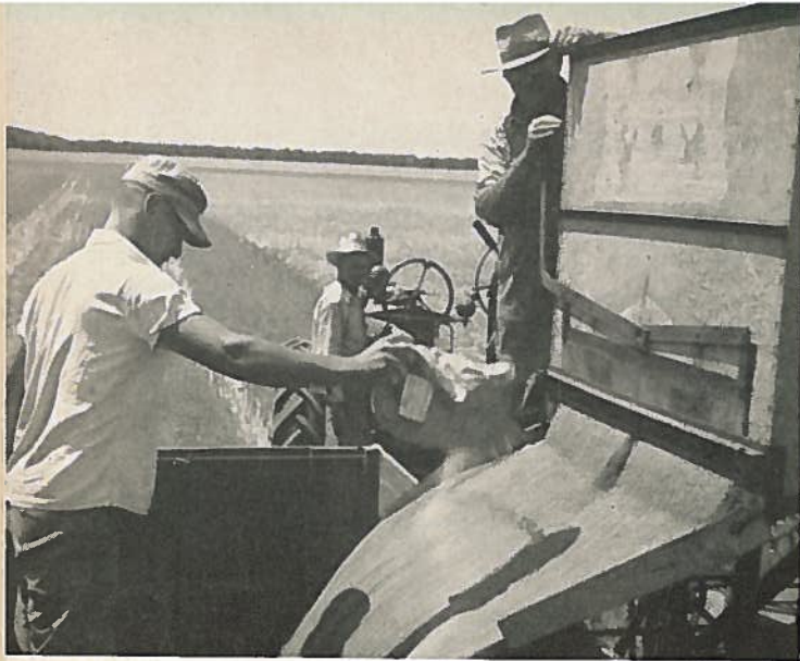
Fig. 10. Applying a protective powder to wheat as it flows from the combine hopper to the truck.
