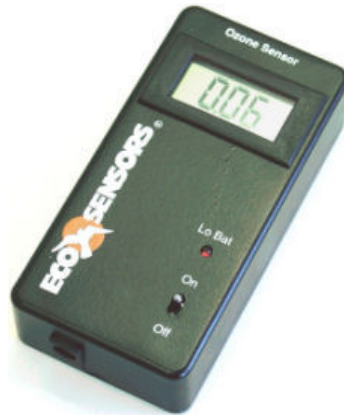
Figure 2-10 Eco Sensors A-21ZX ozone monitor used for monitoring ozone levels in the test environment
