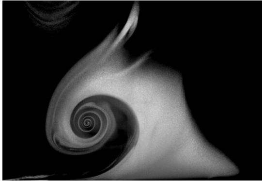
Figure 1-19 Flow visualization showing starting vortex 120 ms after plasma initiation (Whalley and Choi, 2010)
