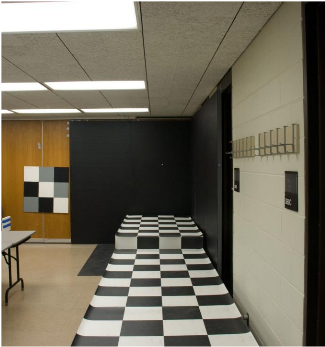
Figure 2.3. Photo of the test space, with the sidewalk and Step Up target covered by textured surfaces. The overhead lighting is also shown.
