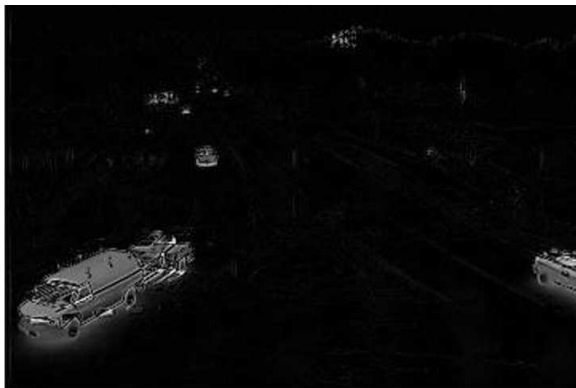
Figure 7: Failed background subtraction. (7a and 7b the raw and thresholded result); Normal background subtraction (7c and 7d the raw and thresholded result)
