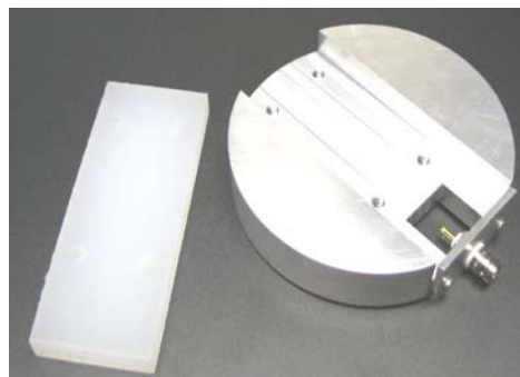
Figure 4.3 Photograph of final design of the sensor platform with replaceable sensor mount (white rectangle) removed from the overall system and placed to its left. This design allows for the sensor to be field replaceable in the event of mechanical or electrical failure, or when sensor designs with improved response are developed.
