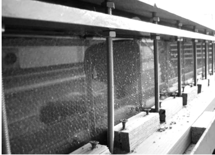
Figure 84. Threaded rod clamping heat exchanger assembly to the channel.
