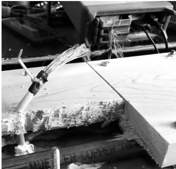
Figure 83. Thermocouple wires routed through heat exchanger to data acquisition unit.
