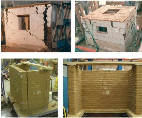
Images: Typical seismic failures produced in adobe structures simulated in physical test.
