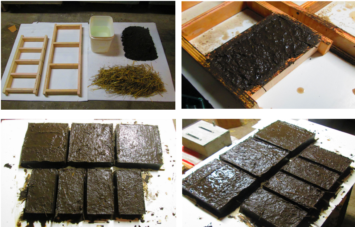
Model in process step 2: Construction of the adobe blocks.
