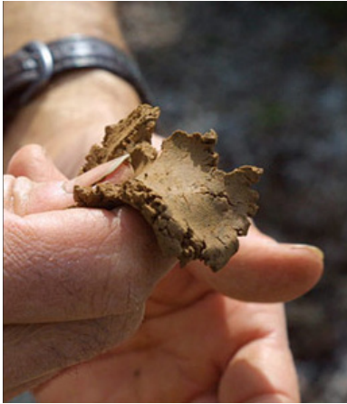
Images: cohesion test. Source: Work Shop School GTZ, Cobquecura 2010. Chile. http://cobquecura.wordpress.com
