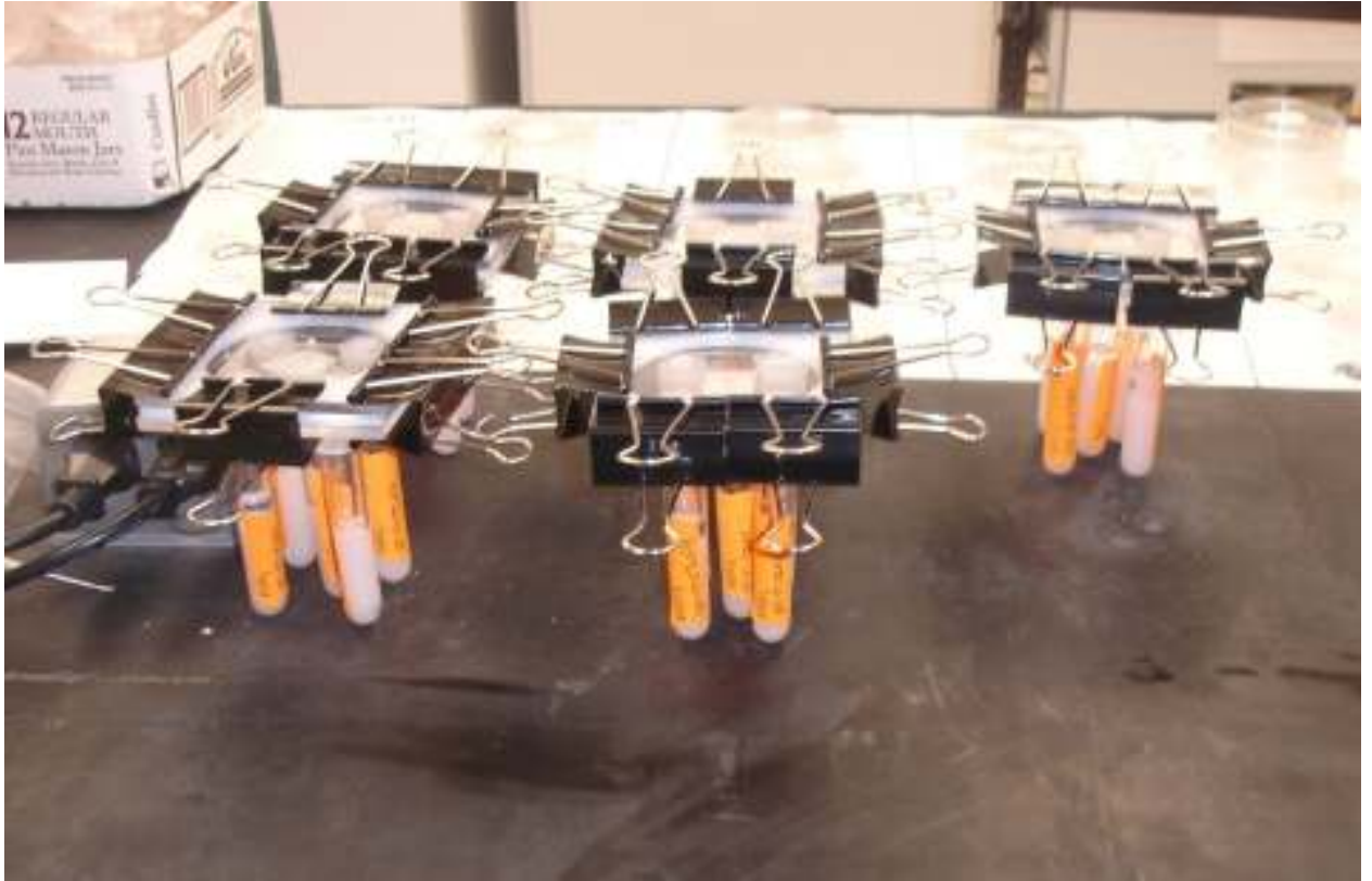
Figure 1. Photograph of assembled humidity arenas. Arenas consisted of two clear cast acrylic plates with a high-density polyethylene (HDPE) plastic layer in between. A hole in the HDPE layer provided the arena walls. Tubes underneath the arena provided a means to adjust humidity using saturated salt solutions.
