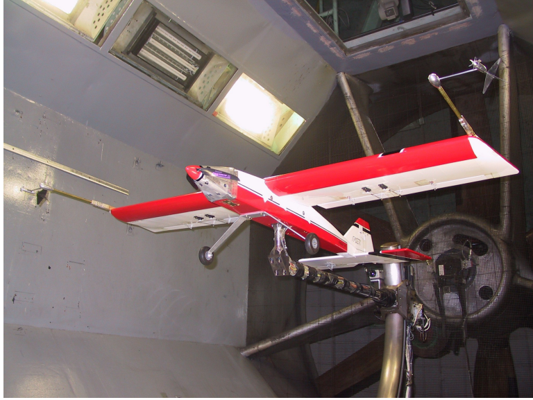
Figure 2.1: FASER mounted in the 12-Foot NASA LaRC Wind Tunnel.
