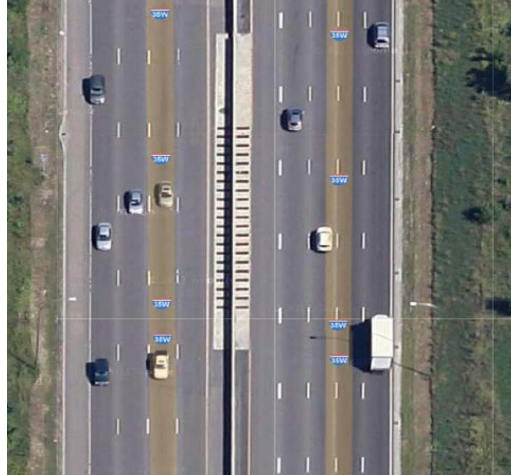
Figure 3.3: Configuration of minor drains (helpers) to reduce runoff bypass.
