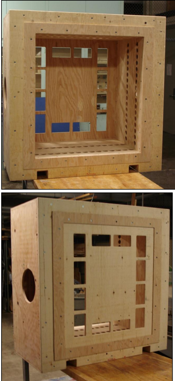
Figure 3.4.1 Turbulence Generator back (top) and front (bottom) taken from Erickson[24] (Refer to Erickson [24] for exact dimensions)
