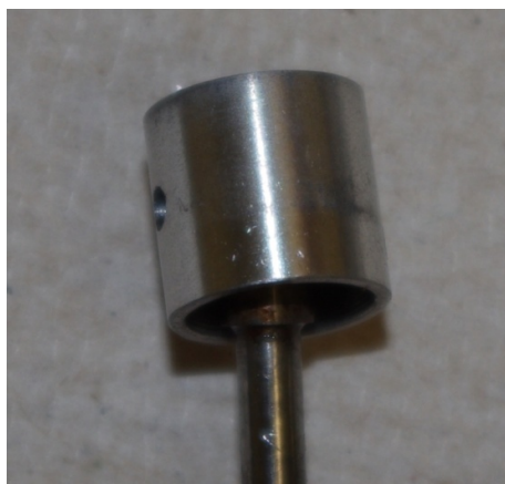
Figure Appx. 7 An evenly worn piston with reamed cylinder liner in prototype
