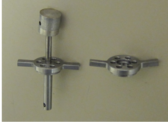
Figure Appx. 10 New (left) and bent (right) connecting rod handles
