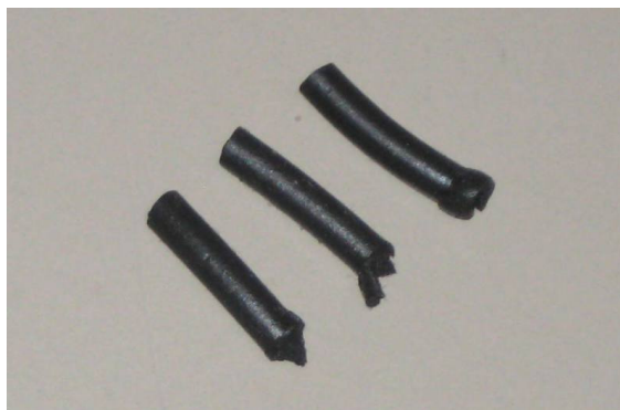
Figure Appx. 11 Several cracked rubber bumper in the prototype
