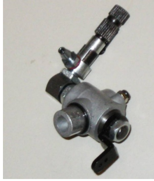
Figure Appx. 9 Model aircraft engine carburetor as used in the prototype
