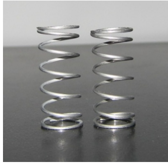
Figure Appx. 13 A new rebound spring (left) and one with 2 minutes run time (right)
