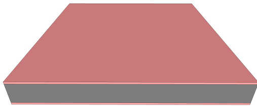
FIGURE 6.1: Model of wafer coated with LPCVD \text{SiN}_x (pink).
