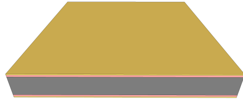
FIGURE 6.2: Model of wafer after ALD \text{Al}_2\text{O}_3 deposition (tan).
