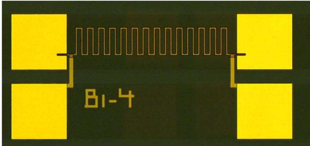
FIGURE 7.9: Test structure for resistivity measurements.
