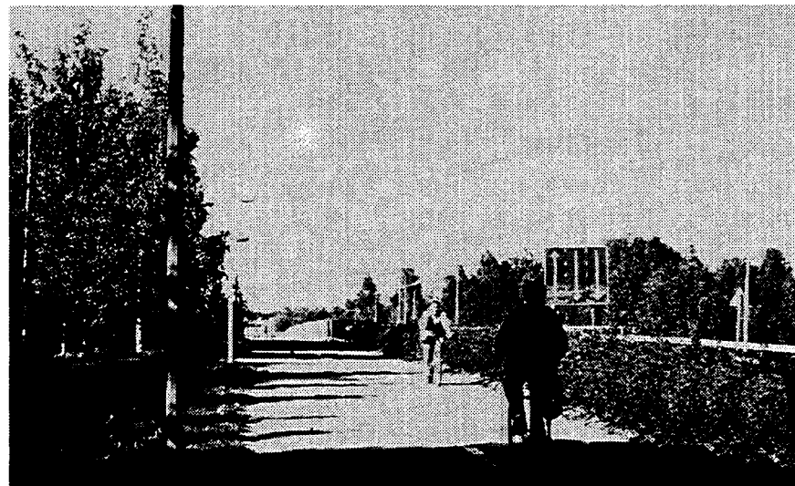
Figure 3-5. Networks of bicycle expressways provide high-speed connections across the city. Bicycle expressways are the most non-stop and directly continuous of all bicycle facilities. They should provide at least two exclusive lanes in each direction.
