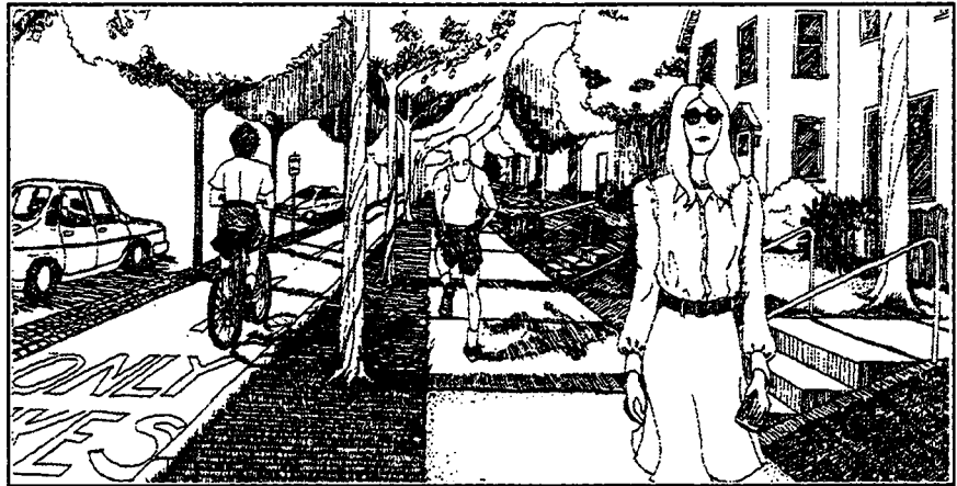
Figure 3-10. Barrier separations physically and spatially separate the bicycle's space with continuous vertical barriers or a series of vertical objects, such as trees, posts, and street furniture.
