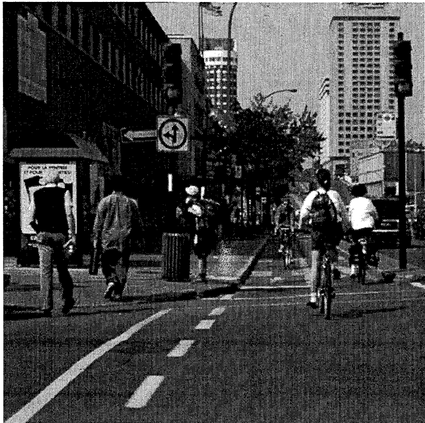
Figure 3-9. Well-designed bicycle facilities can successfully separate bicycle traffic from other uses in the street to create a safe operating environment for cyclists and an attractive street space for everyone.
