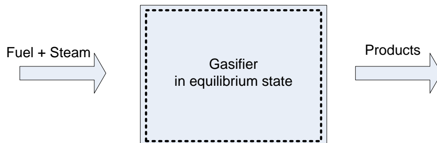
Figure 3. 2 Schematic diagram of the zero-dimensional models modeled as control volume
