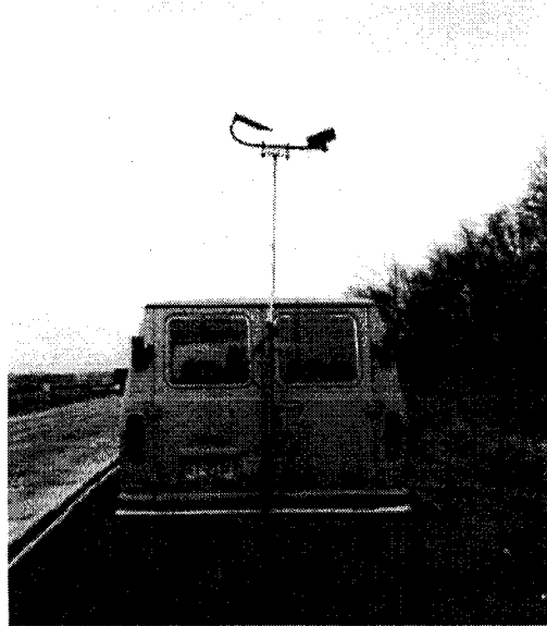
Figure 3.23: Vaisala weather sensor mounted on van
