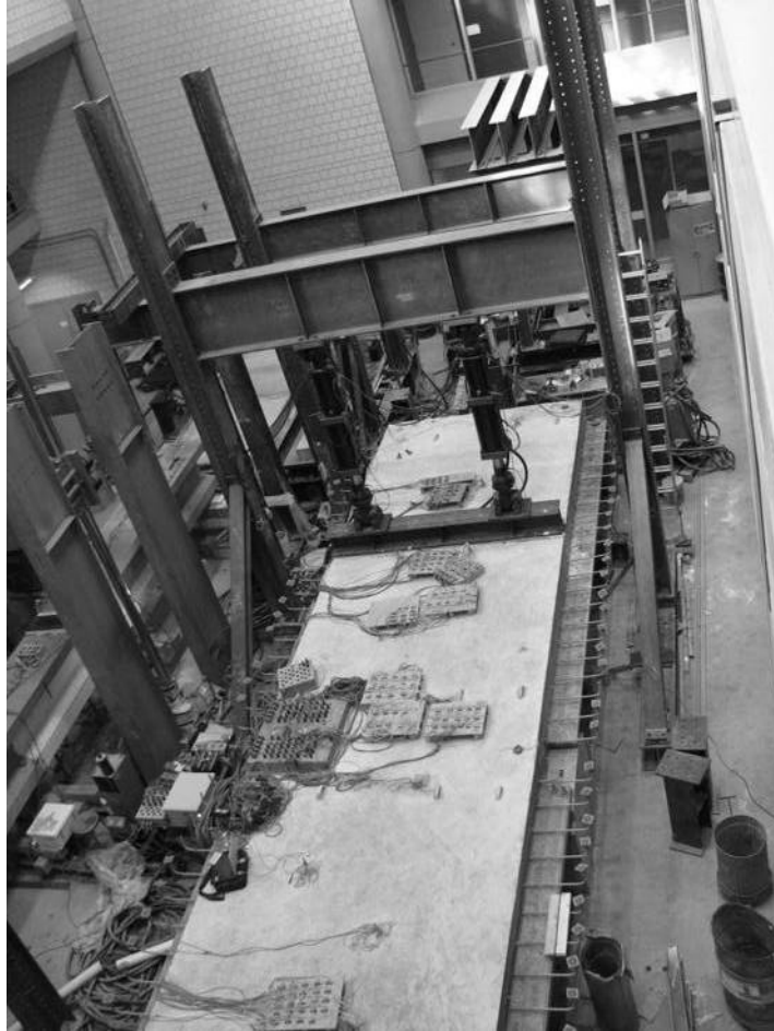
Figure 7.7: Laboratory bridge specimen during spreader beam test of Span 1
