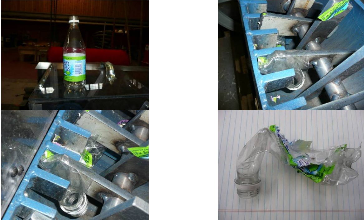
Figure 54: Shredder – plastic bottle
