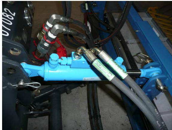
Figure 35: Hydraulic Top Link
