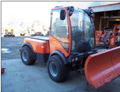
Figure 21: Holder articulated tool carrier
