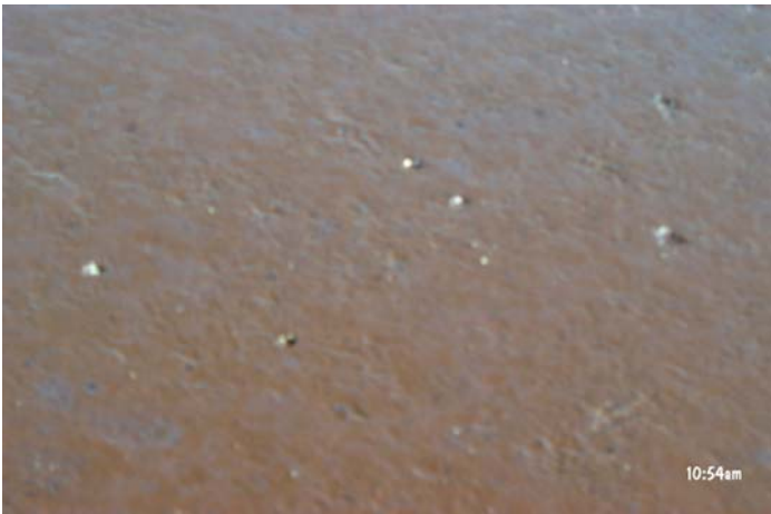
Figure B.8. Emulsion starting to break.
