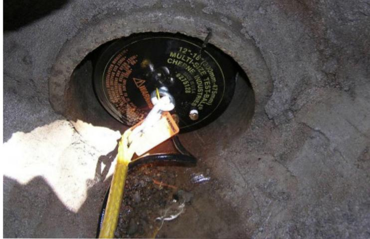
The one-foot-diameter inflatable plug was loaned to researchers by the City of St. Louis Park to control simulated stormwater flow into tested channels.
