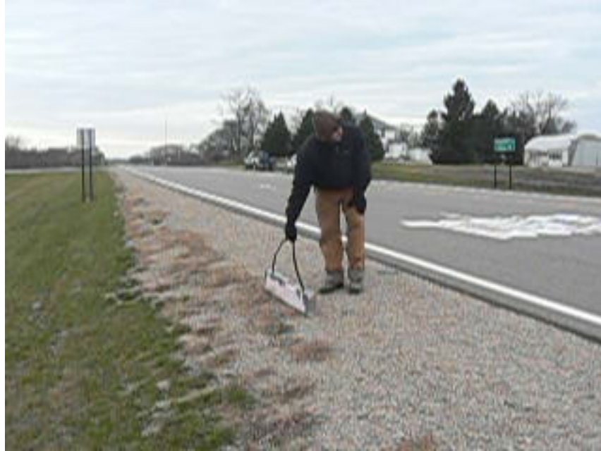
Figure 4.2 Using the EM38 instrument at the CSAH 35 field site
