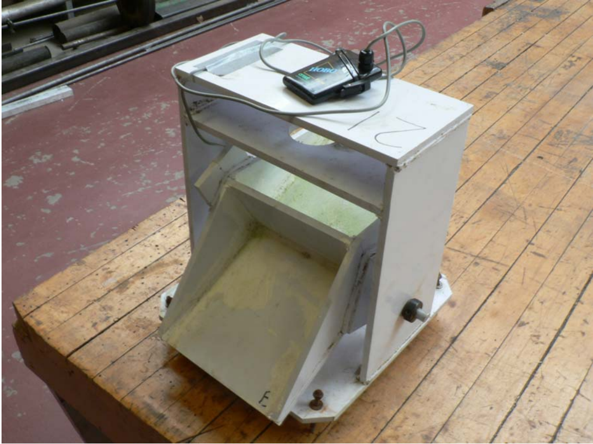
Figure 2.2 A constructed tipping bucket, with a data logger on top of the meter
