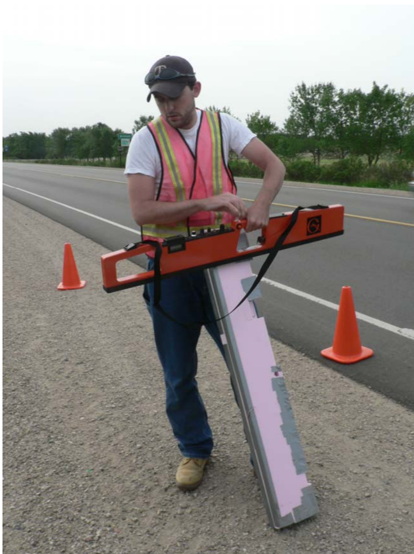
Figure A.13 The EM38 instrument and the insulation enclosure made for the instrument to shield it from environmental temperature fluctuations
