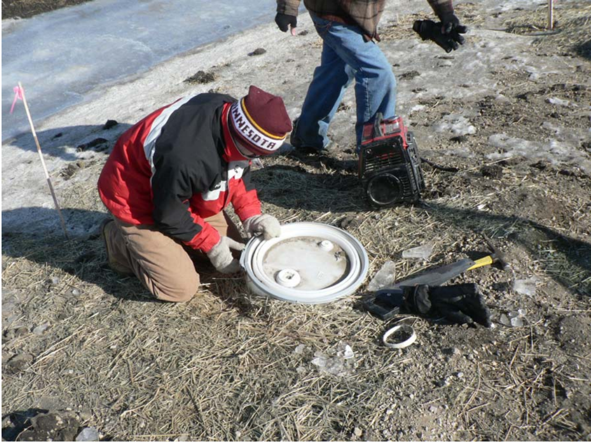
Figure A.6 Closing and the tipping bucket housing. The housing cover is locked to deter vandalism
