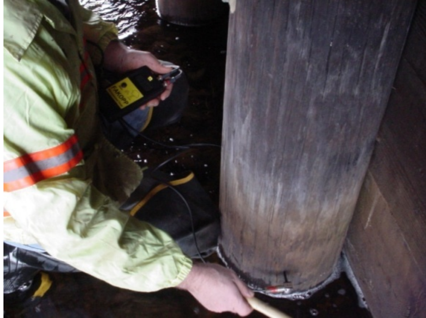
Figure 3.8. Fakopp microsecond timer being used on a timber pile.
