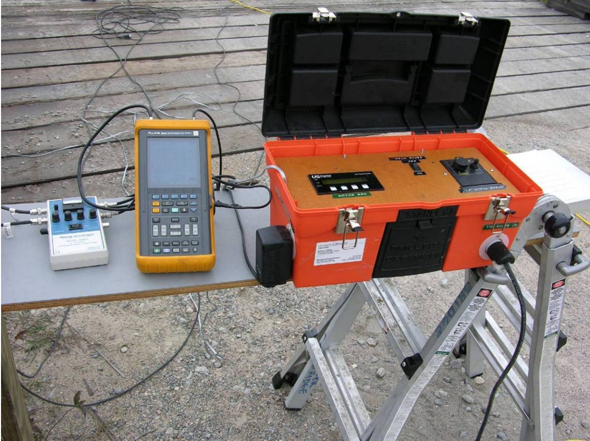
Figure 2.2. Testing system used to control motor and acquire vibration response.
