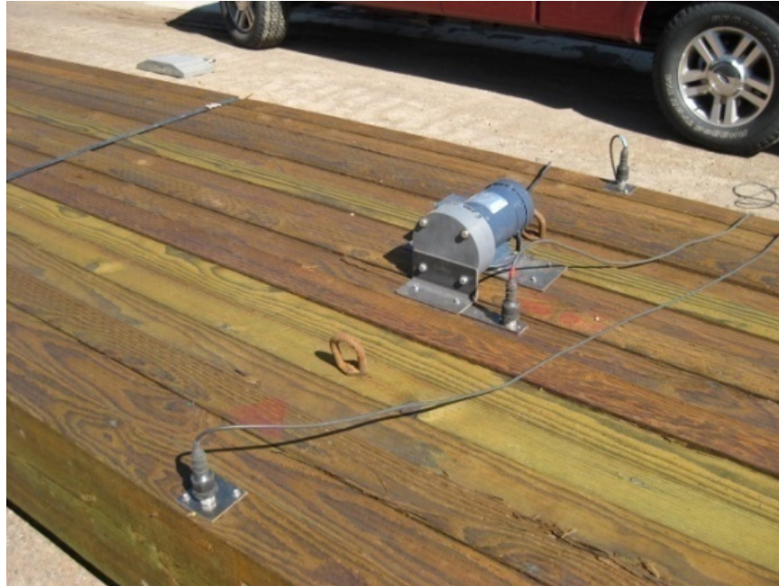
Figure 3.6. General test setup used for vibration testing of each section.
