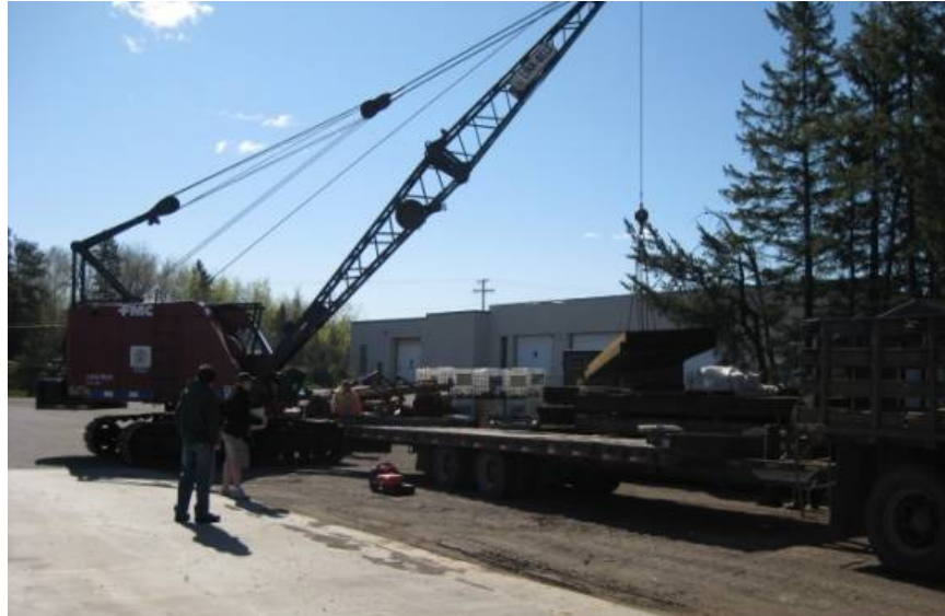
Figure 3.4. The first two tests of the first section were conducted on a trailer. Due to poor signal quality, this technique was abandoned for the remaining testing.
