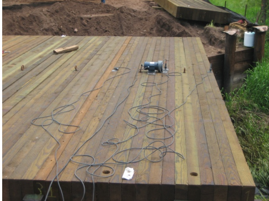
Figure 3.20. The first tests were conducted with the motor in the center of the first section oriented parallel to the laminations.
