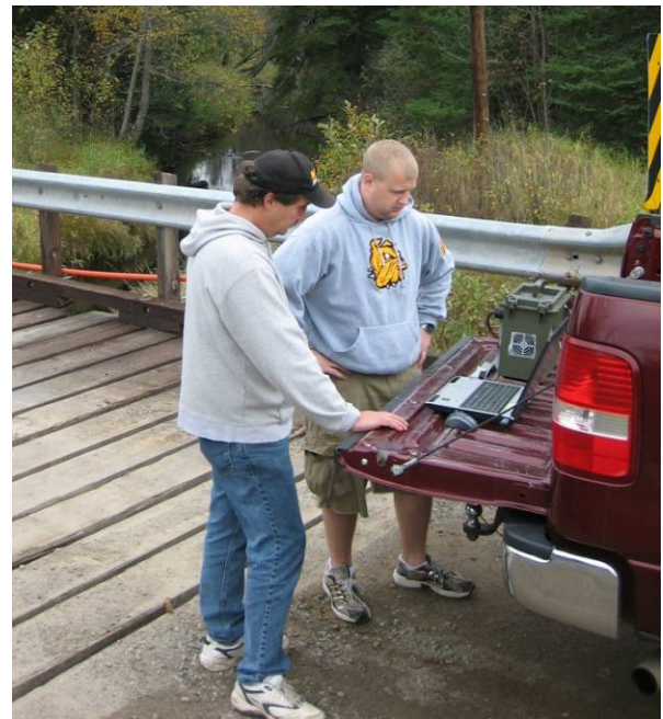
Figure 4.3. Computer controlled interface to control vibration testing and collect vibration characteristics.
