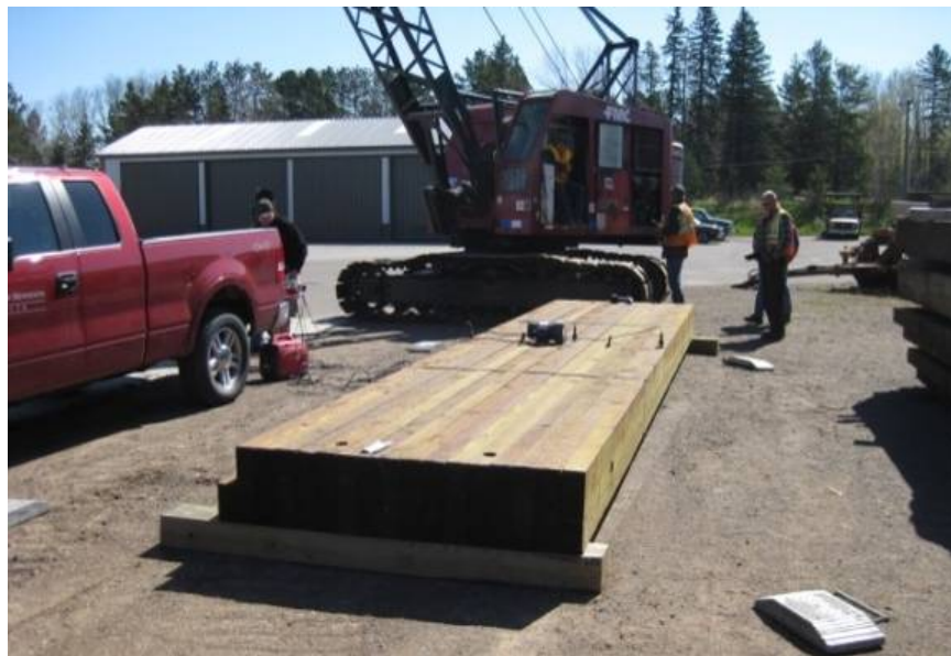
Figure 3.5. The sections were placed on two beams so that they were elevated above the ground for vibration testing.
