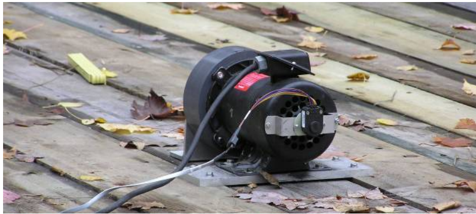
Figure 2.1. Rotating motor used to excite the timber bridge.
