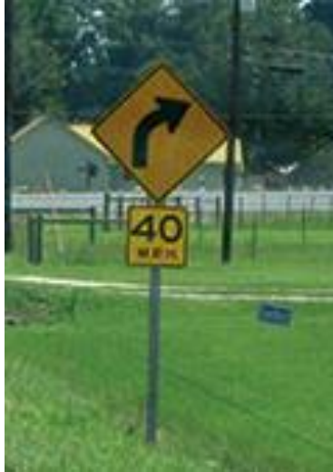
Figure 4.3 Curve Warning Sign with Advisory Speed
