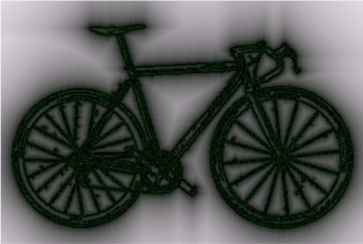
Figure 10: Distance transform template of a bicycle image. Not affine invariant.
