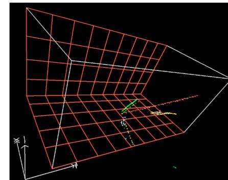
Example 3-D image of an interaction event, using simulated Monte Carlo data in LArSoft. The purpose is to trace the path of interacting neutrinos.
