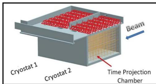
A schematic of the cryostat that make up a 10-kiloton Liquid Argon Far Detector to be located on the surface at the Sanford Underground Research Facility (SURF) in Lead, SD. This is the latest conceptual design for the time projection chamber detector.
