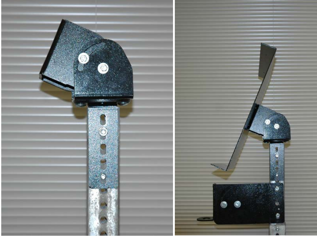
Figure 38: Solar panel mounting bracket (left) and attached solar panel housing (right).
