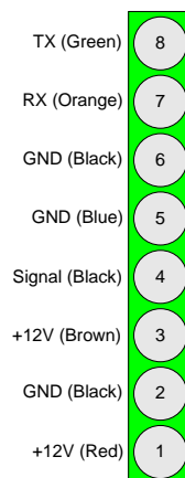
Figure 35: Radar detector 8-pin header.
