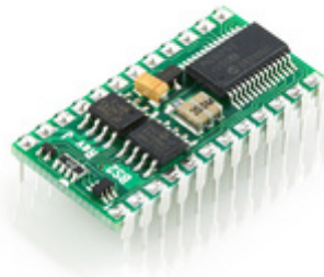
Figure 3.10 Parallax STAMP Microprocessor
