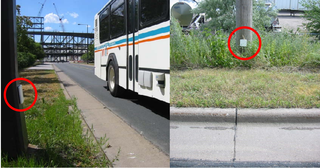
Figure 22. RFID tags placed along the transitway (circled)
