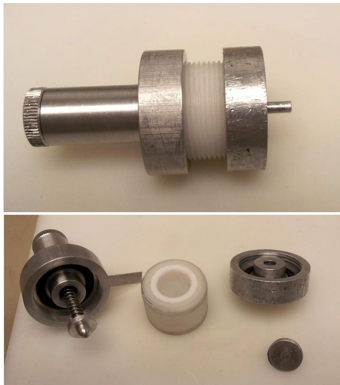
Figure 4.16 Photograph of supercapacitor cell components.
