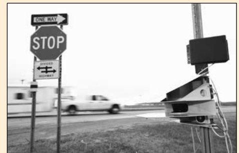
An intersection assistance system deployed at a Minnesota site
