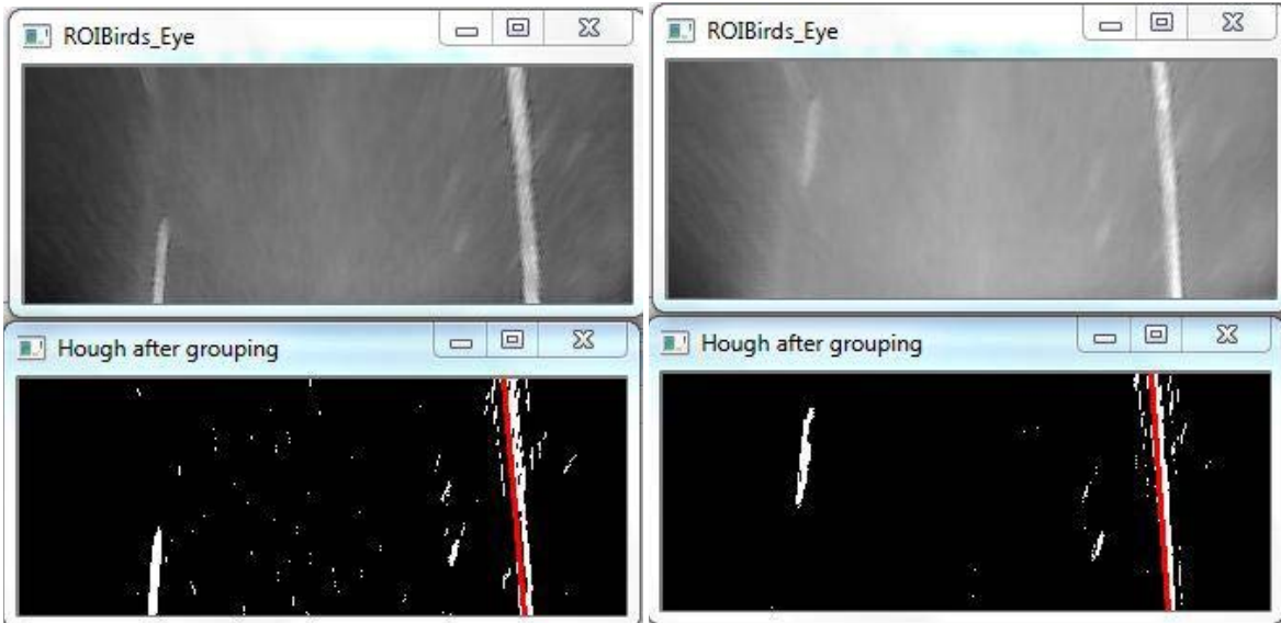
Figure 4.23: Lane markers shown after performing the Hough transform.
