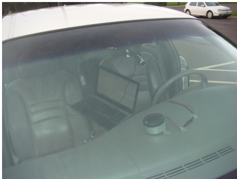
Figure 3.7: The LDW system with the camera and alarm speaker shown.
