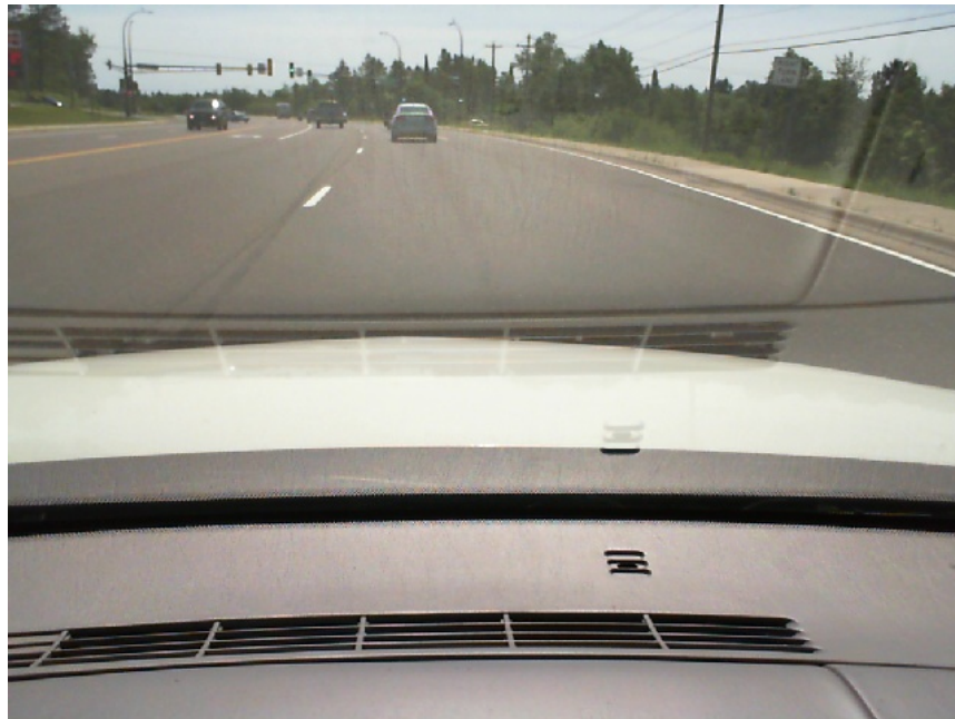
Figure 4.4: The front-view image captured at frame 114 where the left lane marker not available.
