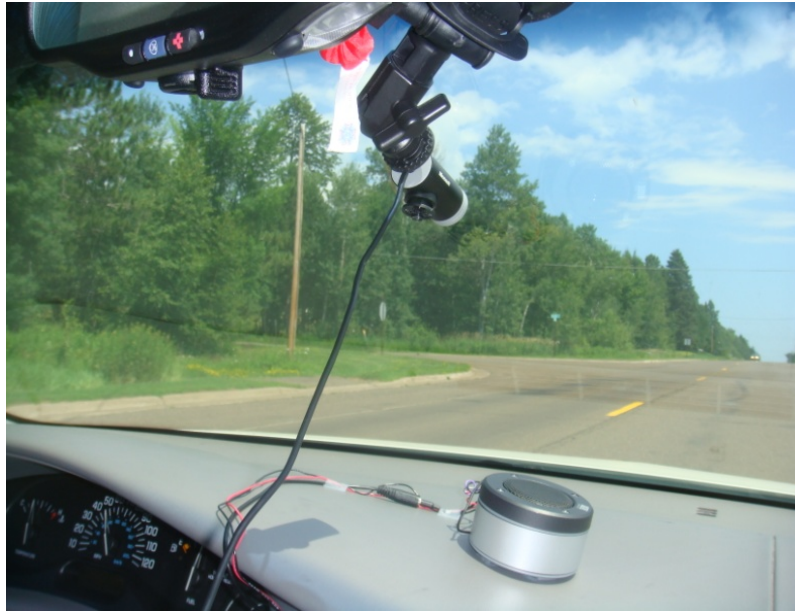
Figure 3.6: The LDW system showing the in-vehicle camera and alarm speaker.
