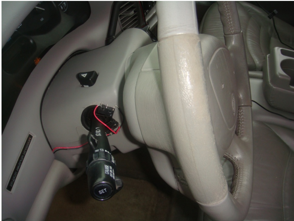
Figure 3.5: Part of the LDW system showing the two switches connected with the turn signal control.
