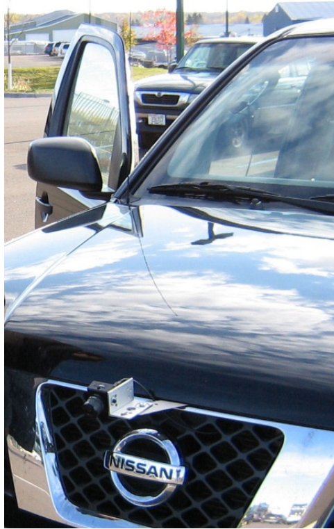
Figure 2.3: Vehicle with camera installed.
