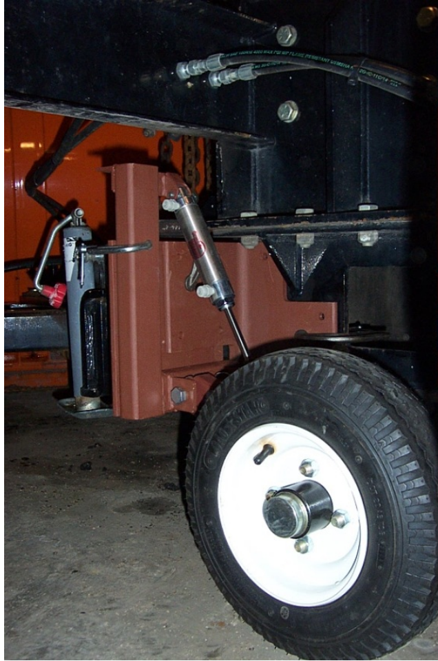
Figure 2: Road friction sensing wheel being installed on a Hennepin Co. snowplow
