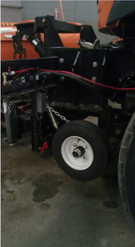
Figure 5: Installed road friction sensing system
