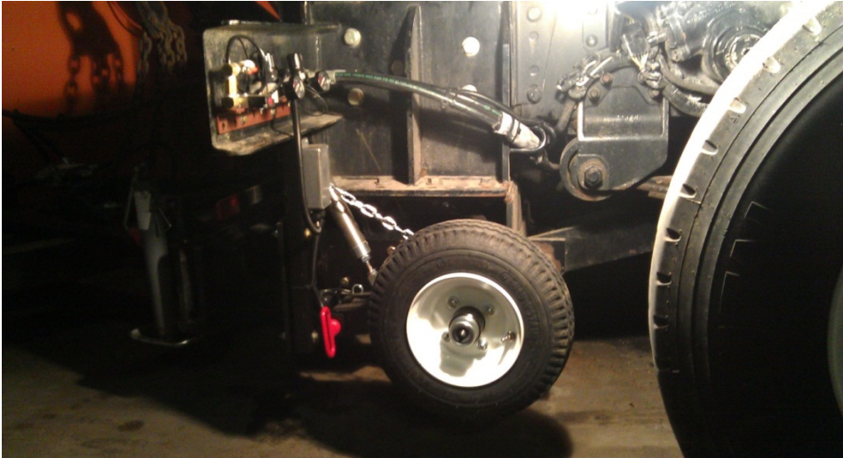
Figure 4: Installed road friction sensing system
