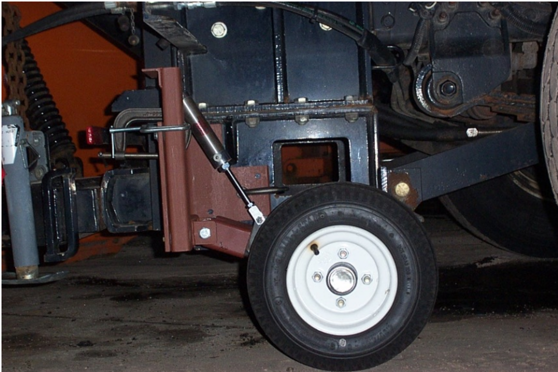
Figure 1: Road friction sensing wheel being installed on a Hennepin Co. snowplow
