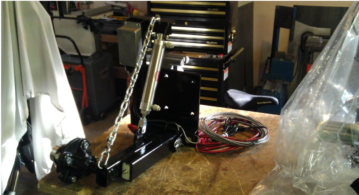
Figure 3: Fabricated road friction sensing system (without wheel and tire) ready for final installation
