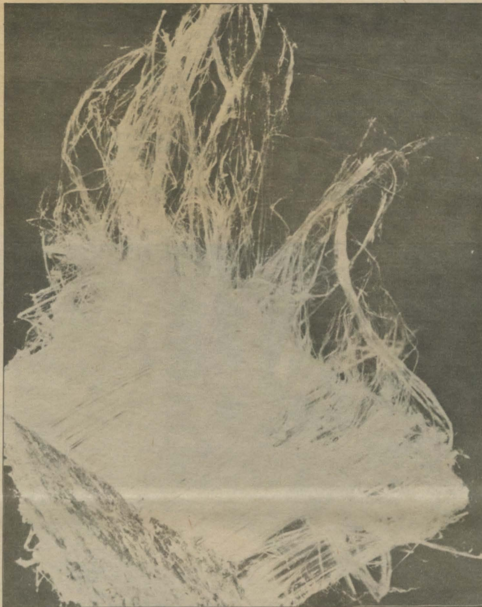
Chrysotile asbestos—interesting to look at, deadly to breathe
