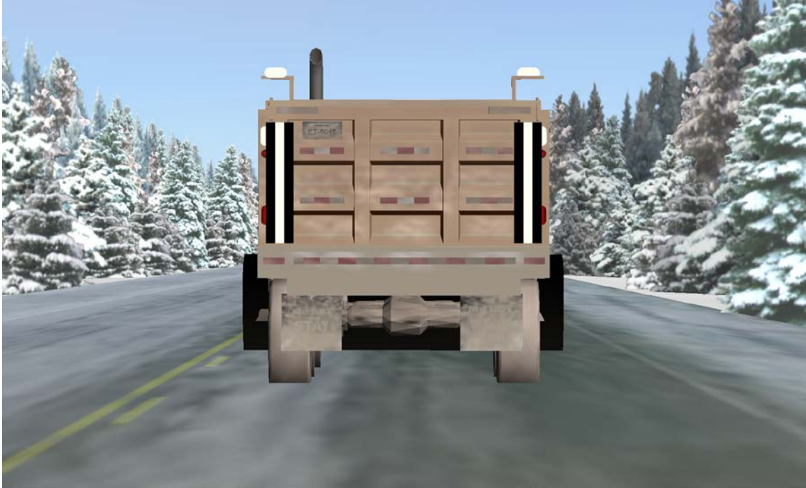
Figure 3.14. Image from the Experiment 4 simulation showing a snowplow truck with rear-end configuration lighting. The lighting configuration attempts to make placement of the light array on the rear of the snowplow more plausible than previous designs. The vertical bar lights are steady burning light arrays flanked by dense black bars to enhance and maximize contrast.
