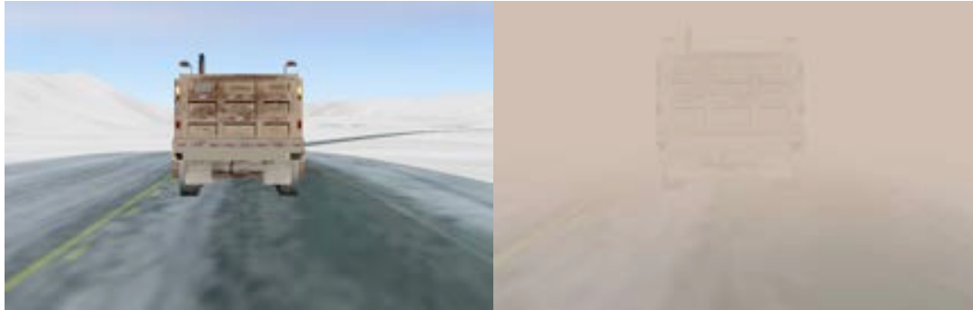
Figure 3.7. Experiments to test the effectiveness of lighting configurations on the back of snowplows are piloted with basic low-luminance contrast versus high-luminance contrast conditions. Normal snowplow lighting is used in both conditions. In the second image, the road and snowplow are partially obscured.
