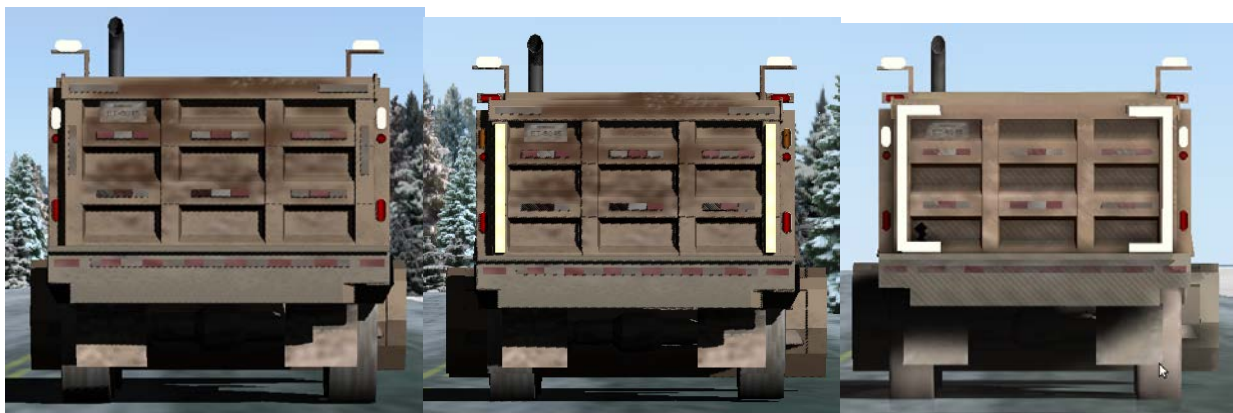
Figure 3.9. Images from the driving simulation showing the different lighting configurations used in Experiment 2. From left to right are the standard snowplow truck lighting, a vertical bar steady lighting, and a vertical bar steady lighting with lighting that adds corners to the vertical bars to frame the back end of the snow plow.
