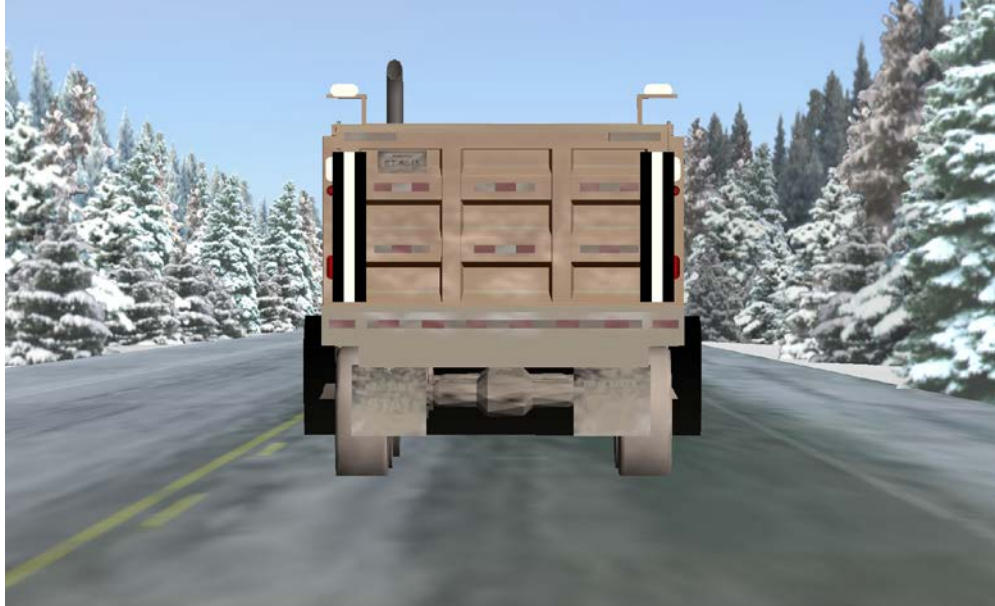
Figure 4.1. Image from the Experiment 4 simulation showing a snowplow truck with rear-end configuration lighting. The lighting configuration attempts to make placement of the light array on the rear of the snowplow more plausible than previous designs. The vertical bar lights are steady burning light arrays flanked by dense black bars to enhance and maximize contrast.
