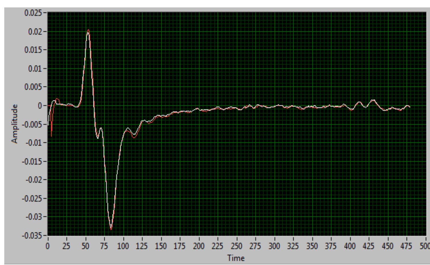
Figure 4: Comparison after sample waveform (Red) has been shifted accordingly to most closely match standard waveform (White), determined by threshold peak heights. Total correlation: 2.97062
