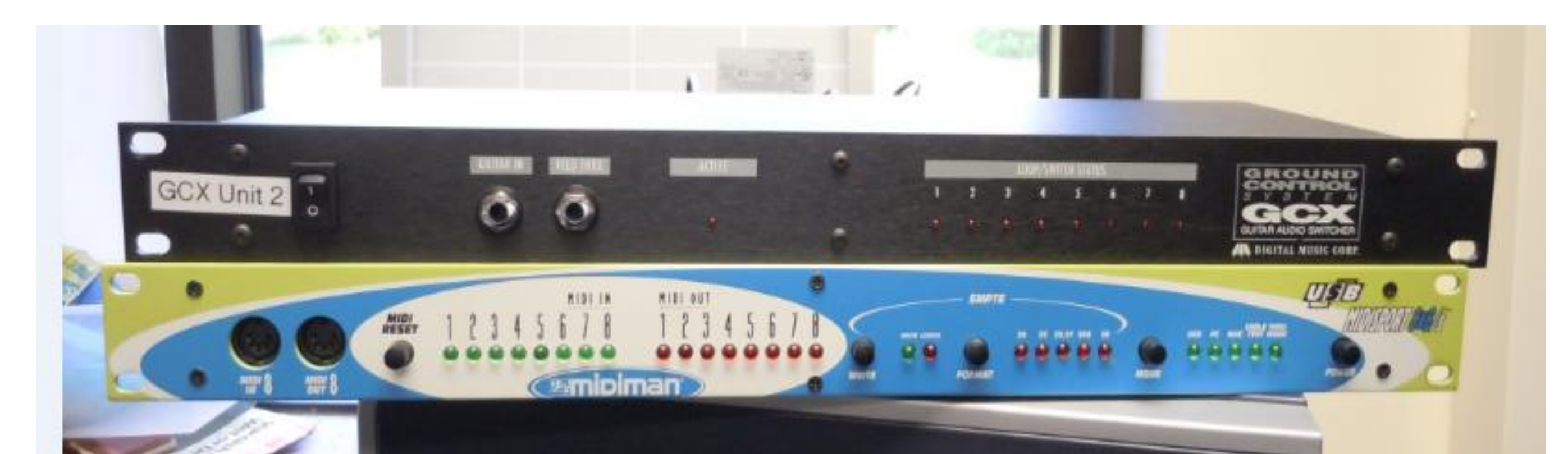
Figure 5: MIDISPORT 8x8/s device (bottom) and GCX guitar audio switcher (top).
