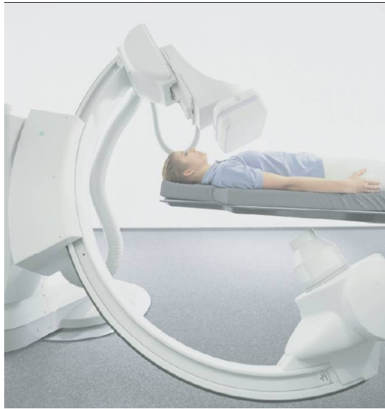
Figure 1.2: A photo of C-arm system. The system has a C shaped arm that can be electronically rotated around a center point (called the isocenter) using a robotic. On one end of the arm is the source that generates the x-ray. On the other end is the detector which is used to generate the image.
