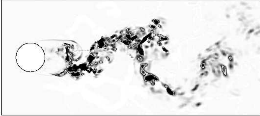
Figure 4.17: Cylinder flow - Re_D = 3900 : Instantaneous contours of Germano-identity error whose contours vary as: 0 \leq (GIE/U_\infty^2)^2 \leq 0.001 .
